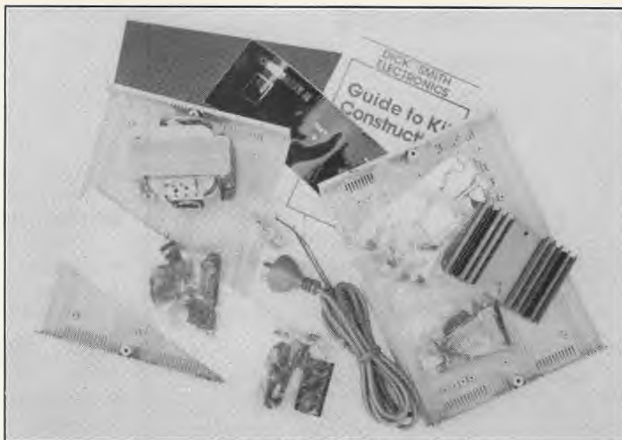
The kit for the D.S.E power supply comes with everything including a substantial transformer, solid plastic case - and comprehensive instructions. Assembly time is around two hours or so.
