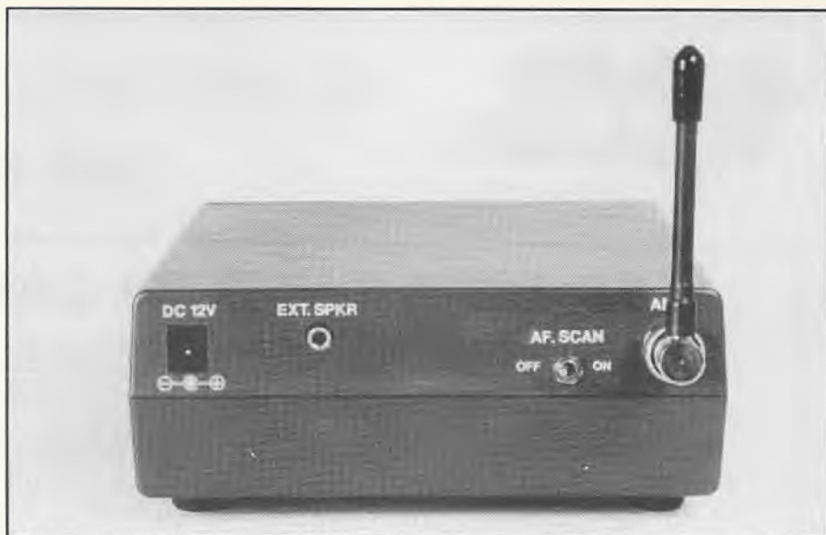
Rear panel has extension speaker outlet, 12V DC socket and AF scan on/off switch plus of course the antenna socket.
