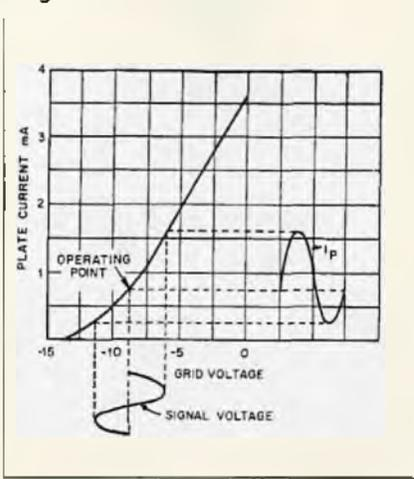
**Figure 6**, known as the *cut-off point*. Now for half the time the valve will operate normally, but for the rest of the time it will not operate at all (ie it will be cut off).
