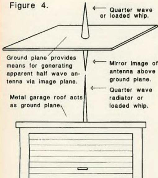
Untuned ground planes should preferably exceed one quarter wavelength radius in all directions from antenna mounting point. Small ground planes usually reduce radiation efficiency and make antenna tuning difficult.
