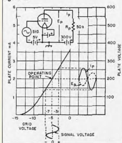
voltage swings back and forth each side of the *operating point*, the plate current varies as shown.
