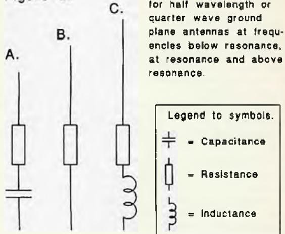
Shortened antenna at 'A' appears resistive with some capacitive reactance in series while antenna at 'C' appears resistive with some inductive reactance in series with the resistance. Antenna 'B' is resonant at the operating frequency and exhibits only pure resistance to the transmitter.
