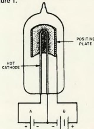
low pressure. In fact, an inert gas is often introduced into the glass bottle, and this helps to determine the electrical characteristics of the valve. Sometimes the term 'soft vacuum' is used to distinguish this situation from a 'hard vacuum', such as in outer space.
