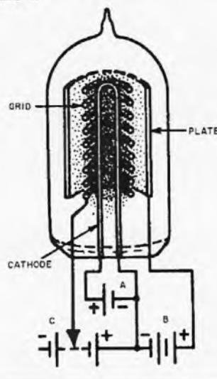
cathode, which has been preventing further electrons from leaving the surface. This means that more electrons will now be able to leave the cathode surface and flow from cathode to anode, thus increasing the current in the device.
