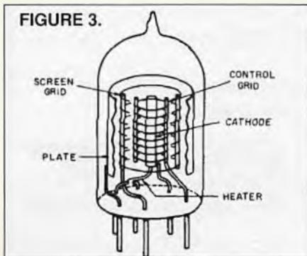
erated by the high voltage on the anode, they are travelling pretty quickly. As they plough into the anode, their energy is absorbed, dislodging a spray of electrons back out of the metal.
