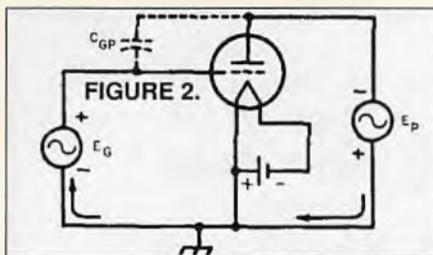
resistor. At high frequencies, the reactance drops to a low value and effectively shorts out the input and output.
