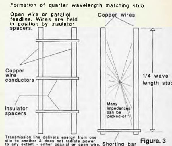
Transmission line delivers energy from one site to another & does not radiate power to any extent - either coaxial or open wire. Shorting bar Figure 3
