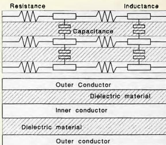
Cross section of coaxial cable above and electrical equivalent top. Figure 2
