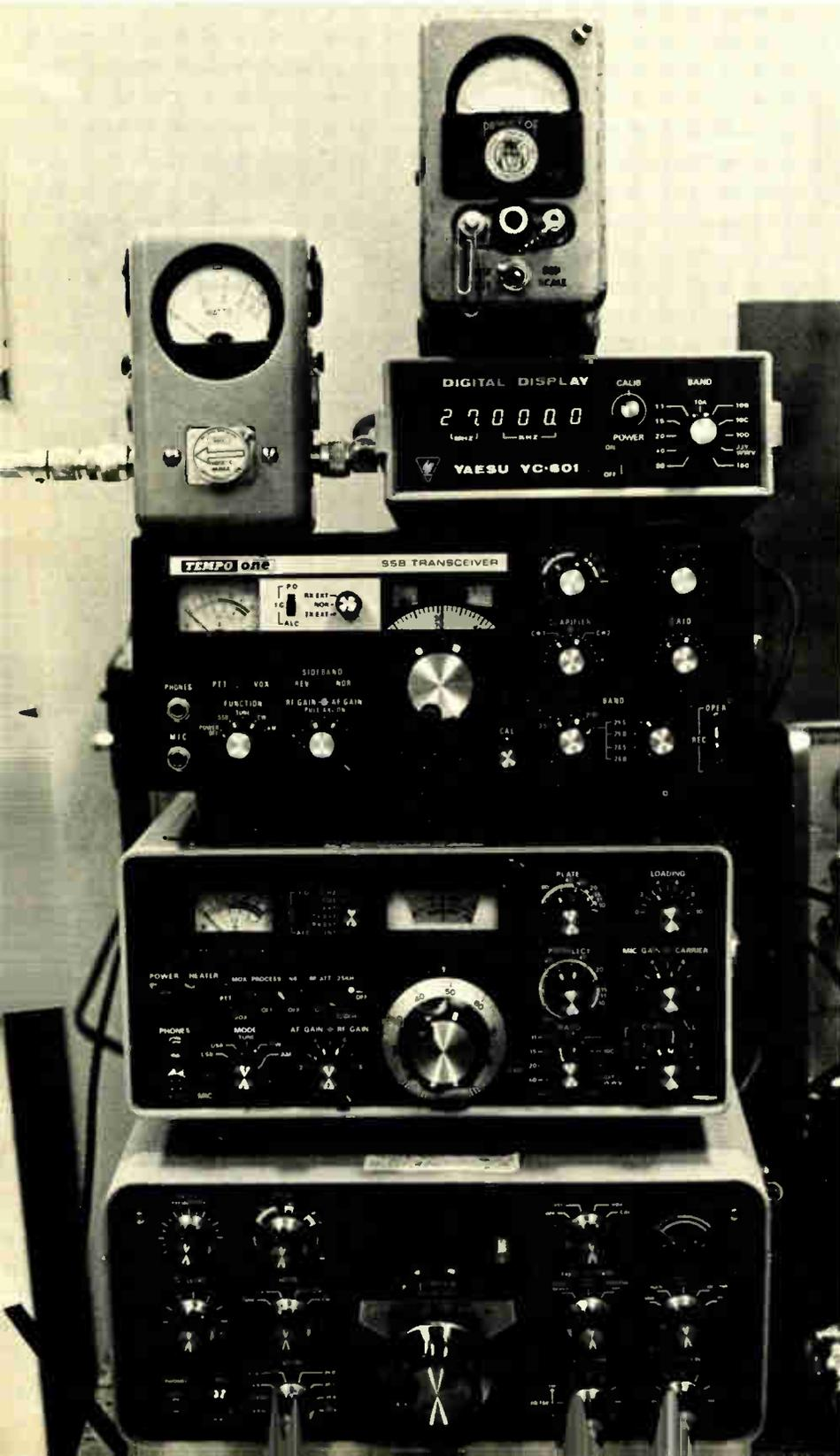
A stack of amateur transceivers which were modified for out-of-band operation. Equipment is being set up for frequency power measurements.
