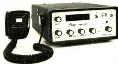
Clegg makes several pieces of gear for the VHF amateur. This synthesized 2-meter transceiver is capable of operating on 1000 different channels.
