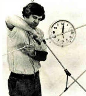
Open like an umbrella....secure ground radials....fully extend bottom radials and tighten.....attach coaxial, slip onto mast and up she goes!
