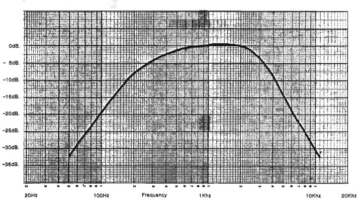
per octave above 3000 Hz. At 10 kHz the response is 30dB down and in terms of transmitter power output this represents only around 0.01 watts from a typical 10 watt transmitter, hardly likely to cause any interference. In practice, the better transmitters will already have some filtering built in and this would reduce the higher frequencies even further.
