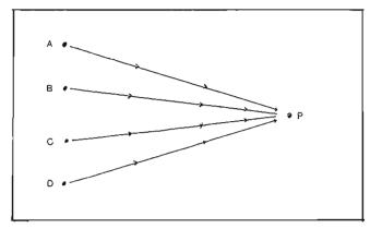
Fig. 1: Radiation from an array of dipoles to a point source (P) See text.
