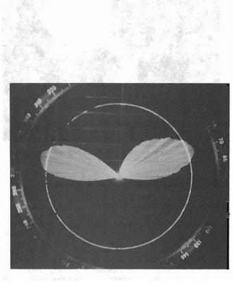
Fig. 6: Vertical angle radiation from a 2 element collinear antenna with gain over a dipole at approximately 2s0. The 'ring' indicates the horizontally omni-directional field. The filin vertical line at right angles to the pottern represents the position of the antenna.
