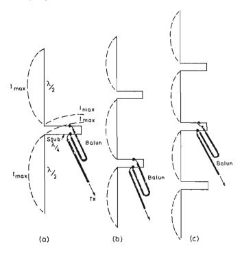
Fig. 5: Electrical configuration of collinear dipole arrays (A) a two element (B) a three element and (C) a four element.
