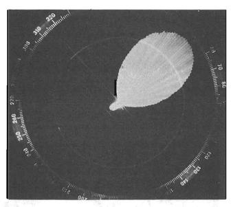
Fig. 2: Horizontal radiation pattern of a typical Yagi type beam antenna.
