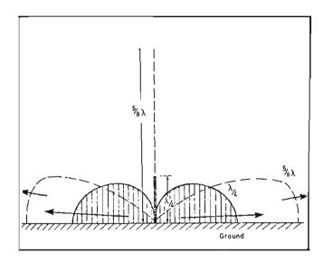
Fig. 3: Theory of the grounded vertical antenna.
