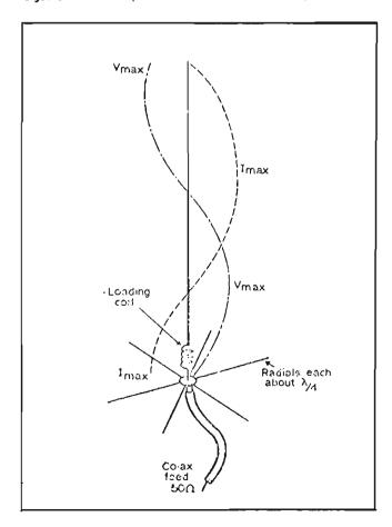
Fig. 4: Electrical configuration of the 5/8 ground plane antenna.
