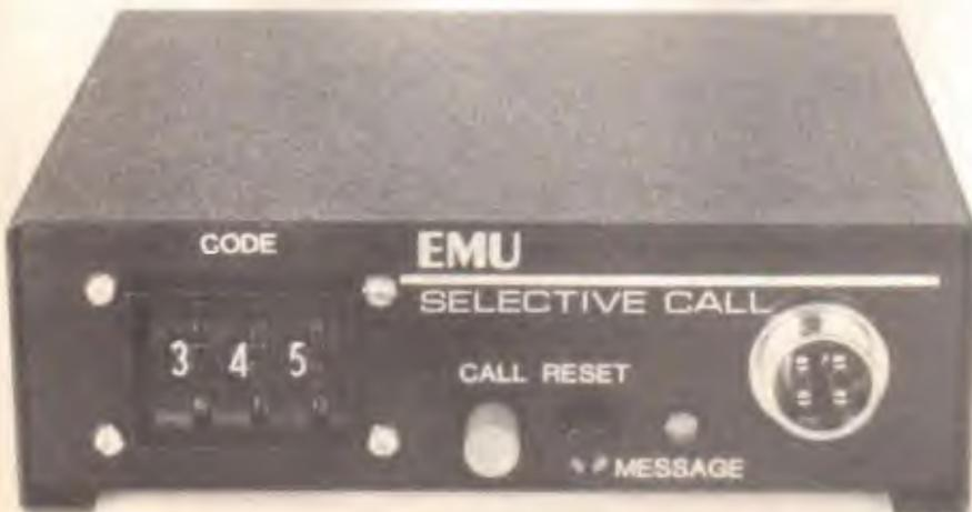
Emu Systems have developed a high-quality sel. call device which can transmit and receive on two different codes, giving greater flexibility when more than two units are used. The receive code is programmed internally and the transmit code selected by three switches on the front panel. The unit also features a message-received light, indicating a call has been received in the user's absence.
