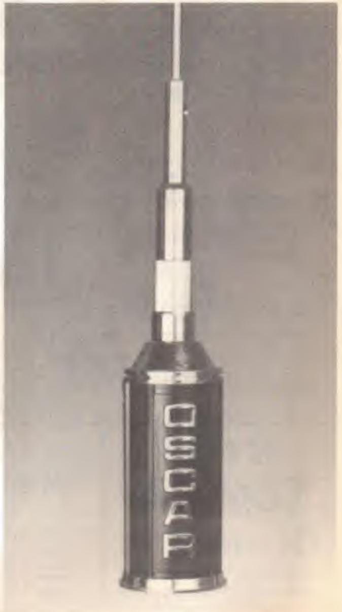
metal fittings. Using a gutter mount the antenna was set up and tuned to resonance at 27.9MHz (band centre) by taking about 1in. off the bottom end of the upper portion of the whip, i.e., the section above the centre coupler. The VSWR readout obtained over the legal FM CB band is shown in Fig. 1.
