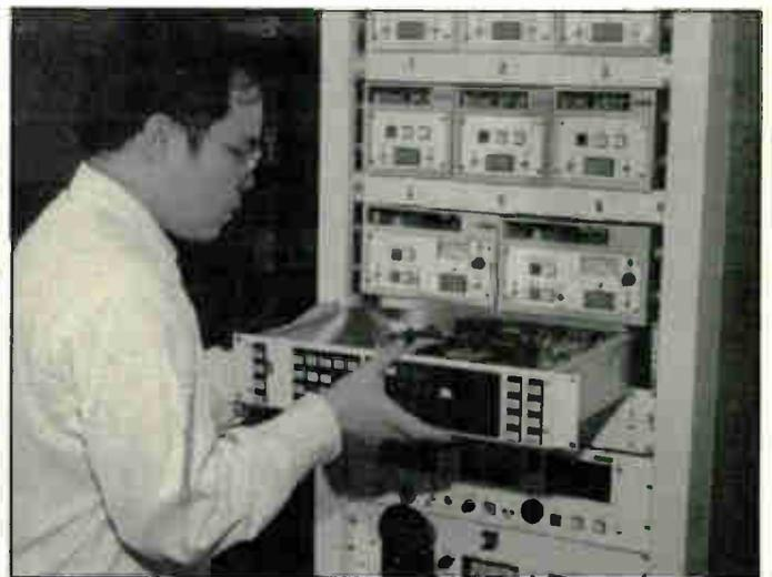
*A National Weather Service technician assembles a new generation of weather radio transmitters which will give the NWS offices new capabilities for broadcasting severe weather watches and warnings to very specific geographic areas, so listeners in other areas won't be bothered by warnings that don't apply to them. (NOAA Photo)*
