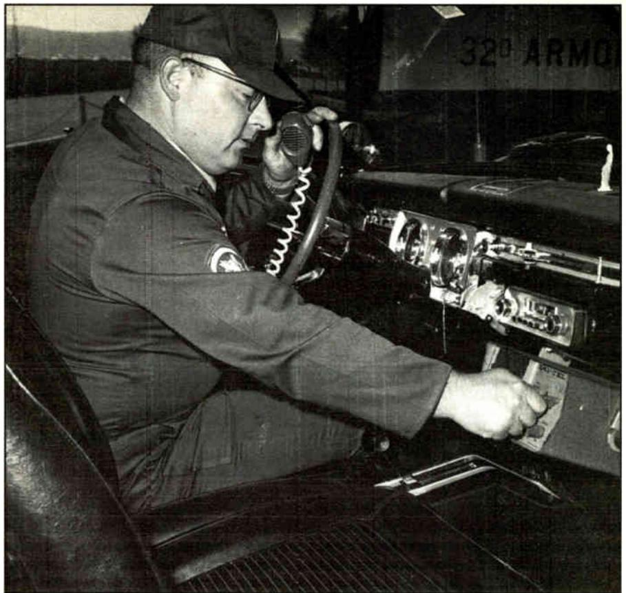
*An bulky vacuum tube CB radio under the dashboard took up much more room than a modern solid state rig.*
