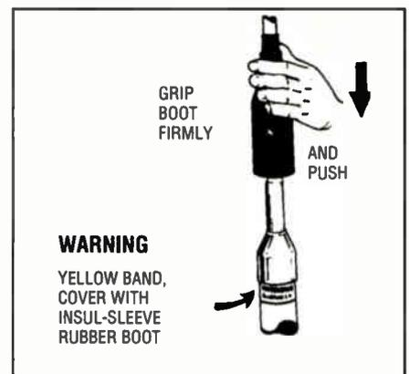
Getting "the boot" to slide down the fiberglass antenna requires a couple of minutes and some patience. Otherwise, the antenna is as easy as 1-2-3 to set up. (Courtesy Shakespeare Electronics, Inc.)
