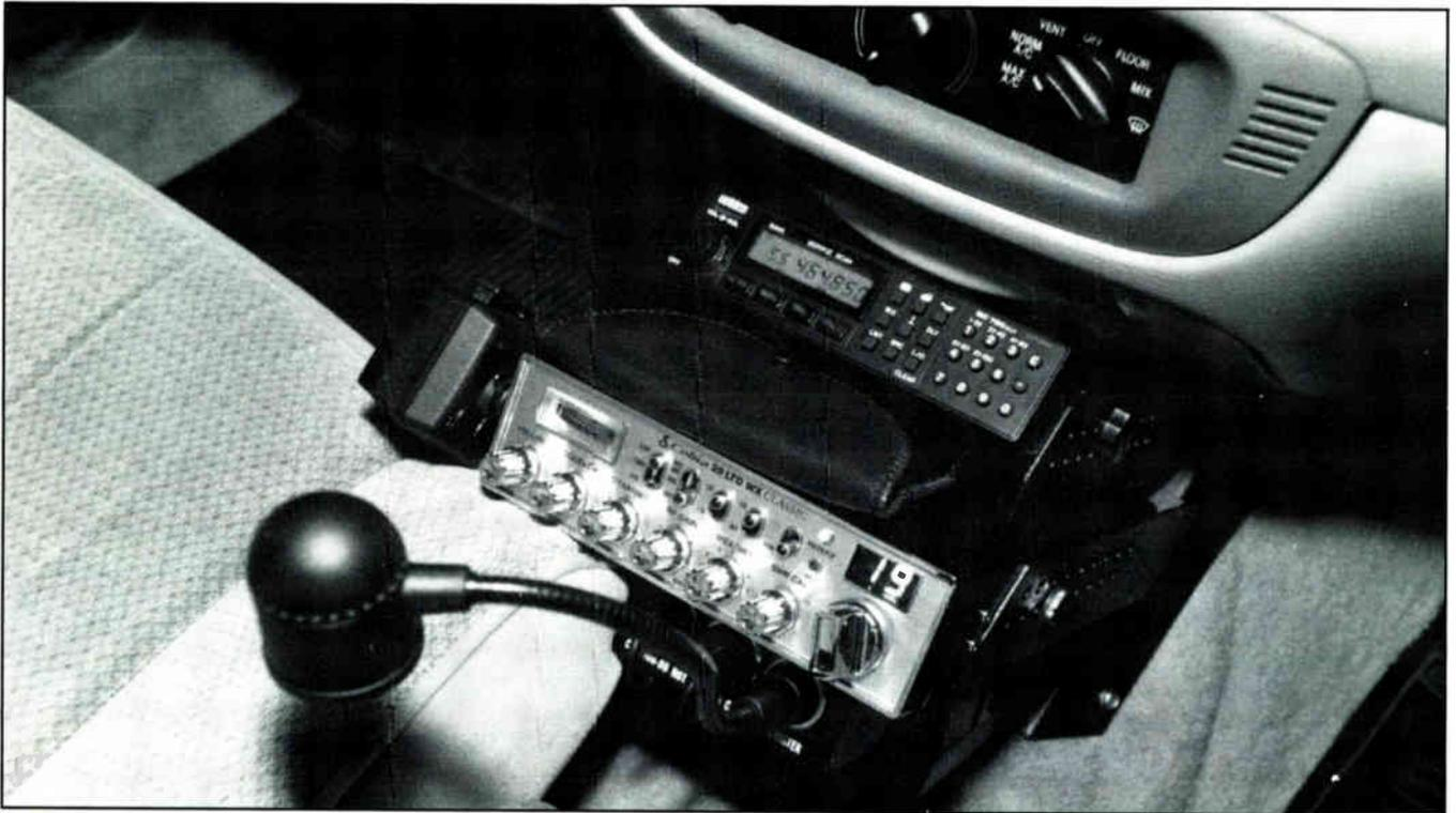
Robin's '95 Crown Vic with his Black Rack, Uniden BC 760 XLT 100 channel scanner, Cobra 29LTD WX Classic CB, Cadet Dash Light, Radio Shack extension speaker, and Gall's three-hole outlet box. You can't see it, but Robin uses an Austin "Spectra" scanner antenna and Larsen NMO 27 low band CB antenna. (Photo by Robin W. Hartford)
