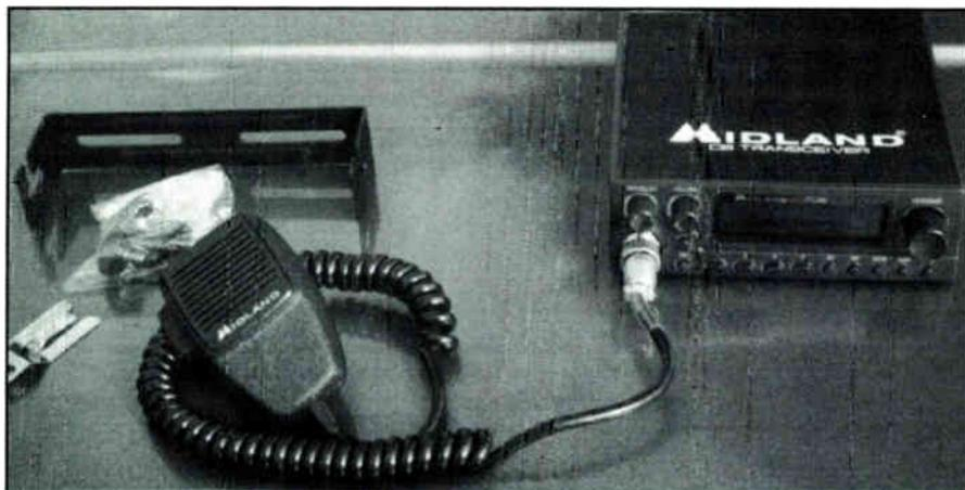
*Getting ready to install the CB; included and well-packaged is the mounting bracket, mic bracket and hardware and power cord. (Photo by Harold Ort)*
