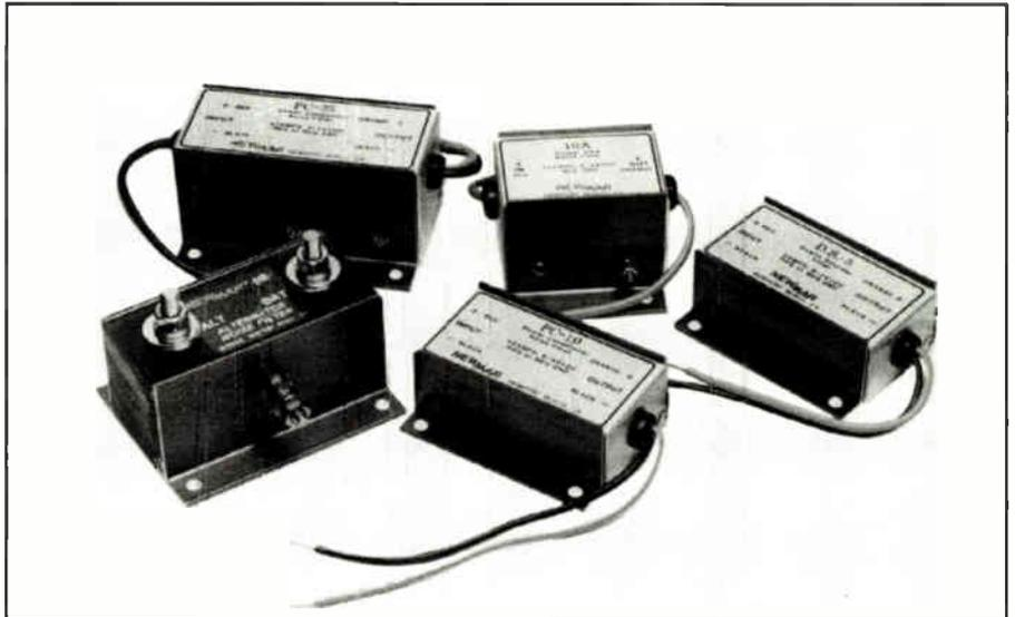
Noise filters are placed next to the interference source in order to stop the racket.
