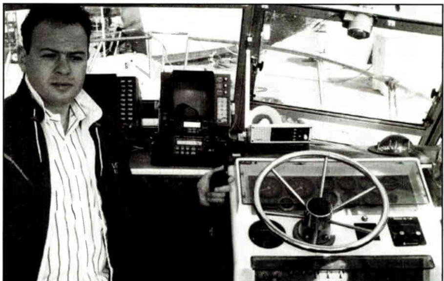
A CB radio (next to the steering wheel) on a boat also needs noise elimination procedures.
