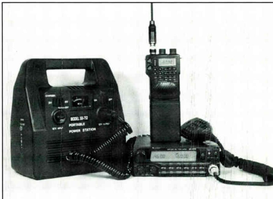
*The Portable Power Station; enough to power a CB walkie-talkie and rig (in this case, though, a couple of ham radios on low power).*
