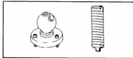
Using a ball and spring mount with the whopping 102-inch stainless steel or fiberglass CB whip antenna will undoubtedly give you the best signal, but it's a monster antenna and requires either drilling a hole in your vehicle or mounting it on the bumper. The spring on the right screws into the top of the ball-mount. Your 102-inch whip screws into the top of the spring.
