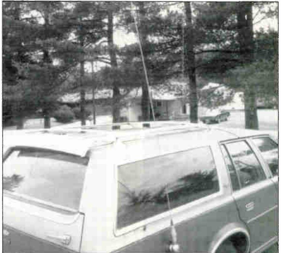
The completed 102" whip on the family vehicle. It's an outstanding performer, but not for everyone. P.S. DON'T mount it on the top of your vehicle—it'll likely hit overhead tree limbs, power lines and garage roofs.
