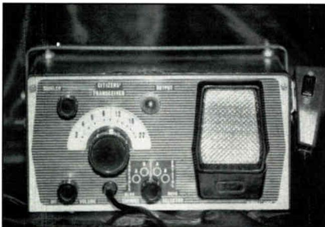
*Electro Voice's RME Model 4305 was a super-het with tunable receive.*
