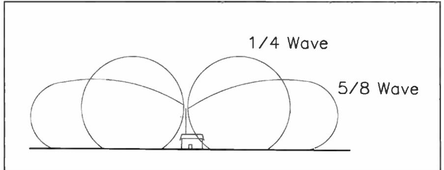
Notice the different radiation patterns between 1/4 and 5/8 wavelength antennas. The 5/8 wavelength antenna puts the radio's signal near the ground, where you want it.
