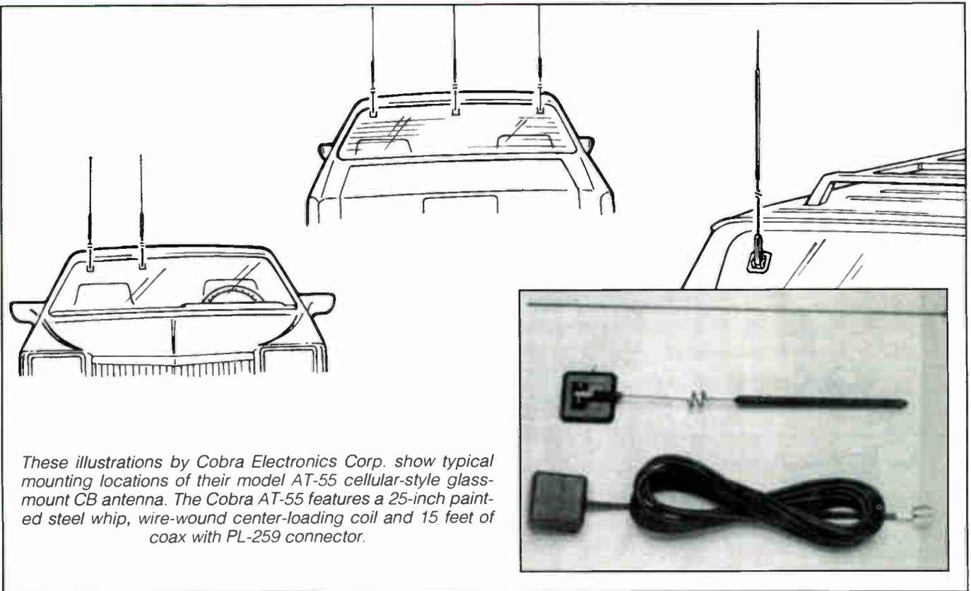
*These illustrations by Cobra Electronics Corp. show typical mounting locations of their model AT-55 cellular-style glass-mount CB antenna. The Cobra AT-55 features a 25-inch painted steel whip, wire-wound center-loading coil and 15 feet of coax with PL-259 connector.*
