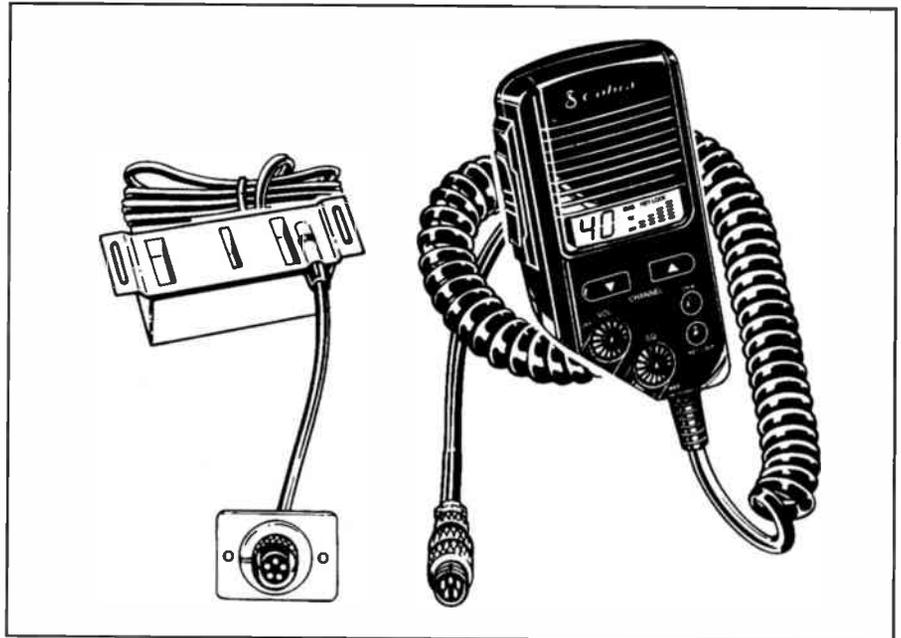
Cobra's HH-70 mobile CB radio allows easy one-hand operation. The CB has a small connector box and two-wire installation. To radio for assistance on the road, a button on the CB switches instantly to Channel 9. The illuminated LCD shows all functions, day or night. It features quick-disconnect for dash or bulkhead mounting. (Courtesy Cobra Electronics Corp.)
