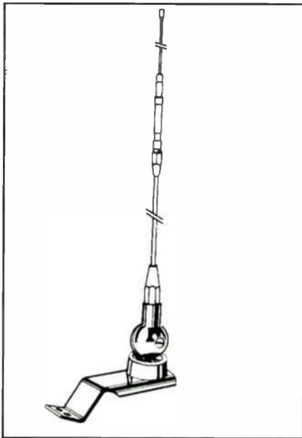
*This trunk or hood-groove mount antenna from Hustler, the TGF-27Ls, is an often-overlooked, but great idea; the antenna mounts inside the trunk/hood groove by drilling two small holes inside the groove. An excellent alternative to the trunk-lip mounts, it's 50-inches tall and includes coax. (Courtesy Hustler, Inc.)*
