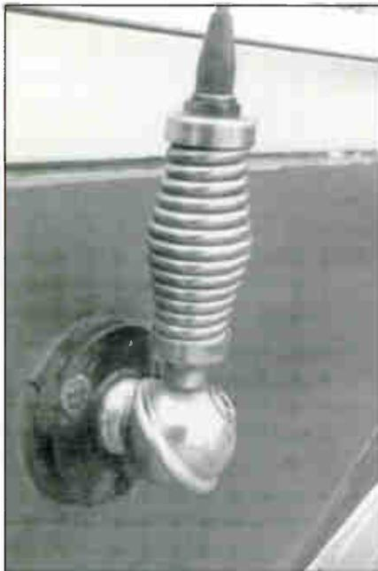
Drilling the hole for the proverbial ball/spring mount to hold your 102" CB whip antenna only takes a minute, but remember, it's permanent! BEFORE you drill, be sure you'll be able to easily get to the inside drilled area; there are three nuts/bolts and coax that must be connected to the assembly. Good planning makes for less holes!
