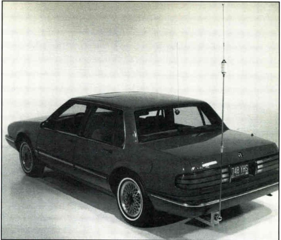
*Still want to use a long whip antenna and NOT drill holes? Fabricating a metal bracket to hold the ball/spring assembly might be the answer. The photo doesn't show close-up detail, you've got to visualize the metal bracket bolted to the car's undercarriage. This connection eliminates drilling a large hole for the ball assembly. (Courtesy General Motors Corporation)*
