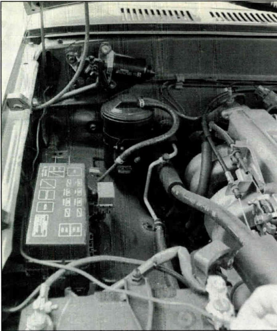
Notice the wire coming out of the fire wall under the hood hinge? That's this CBER's red "positive" power cable running directly to the positive terminal of the car's battery near the front of the photo. (Photo by Bill Price)
