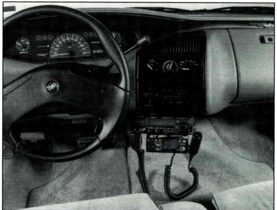
*It worked for GM, but you know as well as I, that once you've drilled the holes, they're there to stay! Be sure to find out what you're drilling through before taking the plunge; piggy-backing a couple of heavy radios, however small, requires a well-planned assembly before the drill bit turns. (Courtesy General Motors Corporation)*
