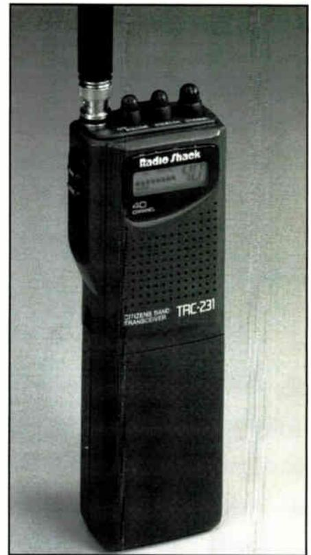
*This RadioShack TRC-231 CB walkie-talkie is ideal for virtually any emergency situation. It is powered by alkaline or NiCd batteries. (Courtesy RadioShack)*
