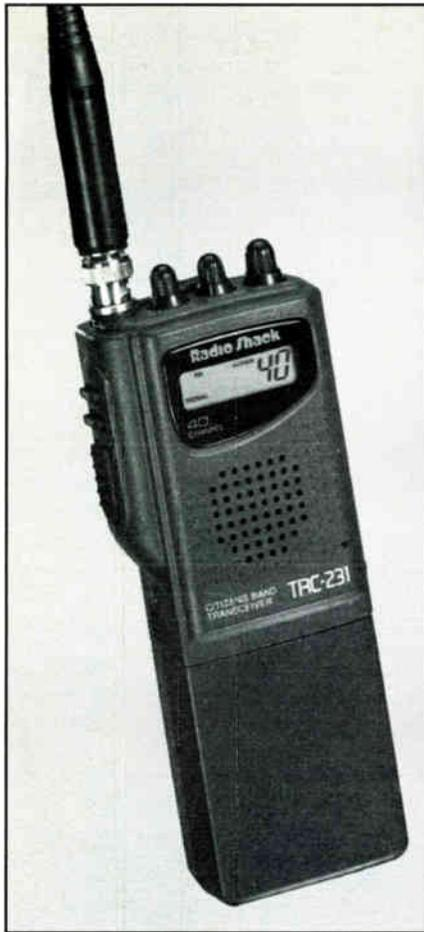
*CB walkie-talkies like this RadioShack model with flexible "rubber duck" antenna are ideal for hiking. (Courtesy RadioShack)*
