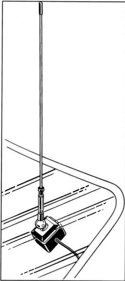
Solarcon's Thru-Glass CB mobile antenna is a half-wave antenna. It's tunable for 10-11 meters and includes 16 feet of coax with PL-259 connector. It's ready-to-go. The 24-inch whip is even removable. (Courtesy Solarcon Antenna Research)
