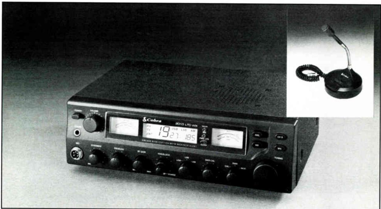
The Cobra 2010 GTL WX is a full-featured base AM/SSB transceiver. (Courtesy Cobra Electronics Corp.)
