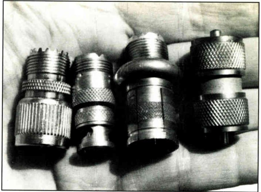
None of the coaxial cable plugs seen here are waterproof. They MUST be sealed.
