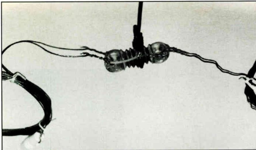
*The center portion of a coiled-up dipole.*
