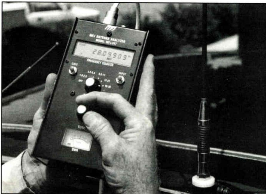
*The whip needs to be lengthened. It's best SWR is at 28 MHz, when it should be at 27 MHz.*
