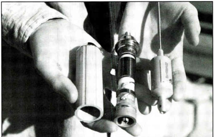
Here's a tapped base-load (left) and center-load on the right.
