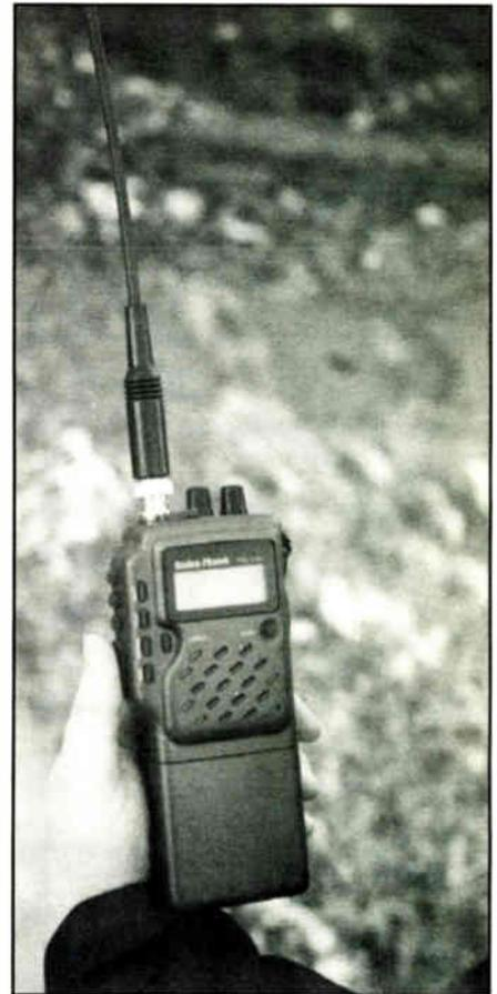
A look at the TRC-232 walkie-talkie with the alkaline battery pack attached. Using the supplied rubber duck antenna it puts out a potent signal, easily giving about 1 1/2 miles unit-to-unit range in a residential area. The professional appearance of the unit is matched by its performance!
