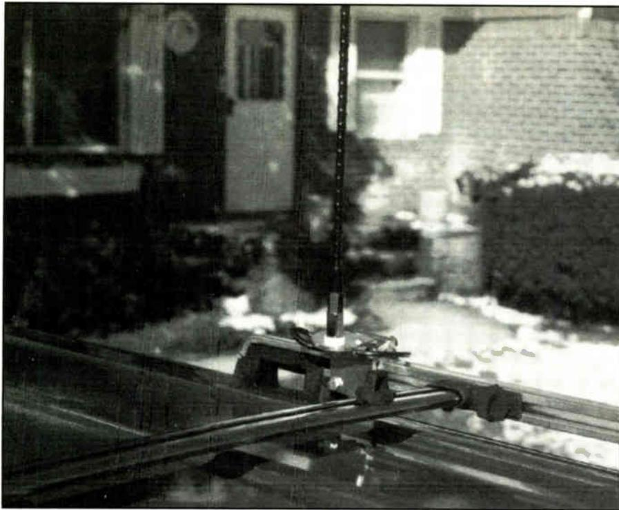
The Marvel NGP-1 mounted to a fiberglass mini-van. Notice the easy-to-use mounting bracket. (Photo by Jim Barry, SSB-930)
