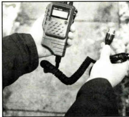
*The RadioShack TRC-232 CB walkie-talkie comes complete with a handy vehicle power/antenna adapter. Simply remove the battery pack from the bottom of the radio, slide on the power adapter, plug in the cigarette lighter cord, connect your antenna, and you're on the air from your vehicle. In this configuration, the radio is only a bit larger than a standard mobile CB mic. The power cord isn't a flimsy cord either, and the plug is even fused.*
