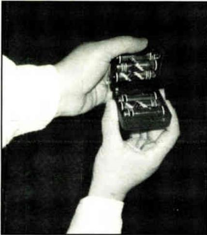
Here's a look at the 6 "AA" alkalines in the battery pack. Always use alkalines or (in the other supplied battery case) NiCds, and NEVER mix types of batteries! We found the battery cases somewhat difficult to open; for this reason we suggest buying NiCds and a charger right away. This way you open the NiCd case once and you're set for a long time.
