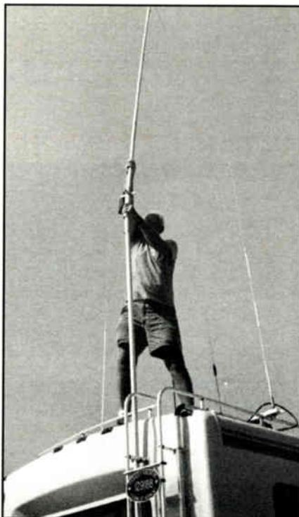
*When a big base CB antenna gets water into it, you must remove it to drain out the water. WATCH FOR POWER LINES!*
