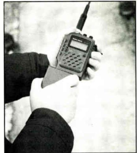
*Unlike the RadioShack amateur HT's, the battery pack on the TRC-232 slides off from right to left. It's a bit awkward, requiring a good grip on the radio portion of the unit.*
