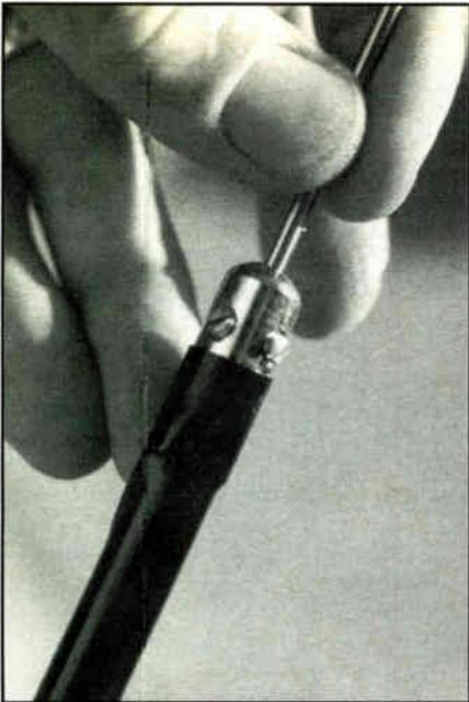
*LENGTHEN the mobile CB whip to LOWER the best SWR readings.*
