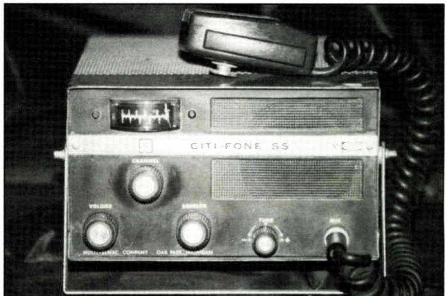
*An older CB radio uses relays to switch from transmit to receiver.*
