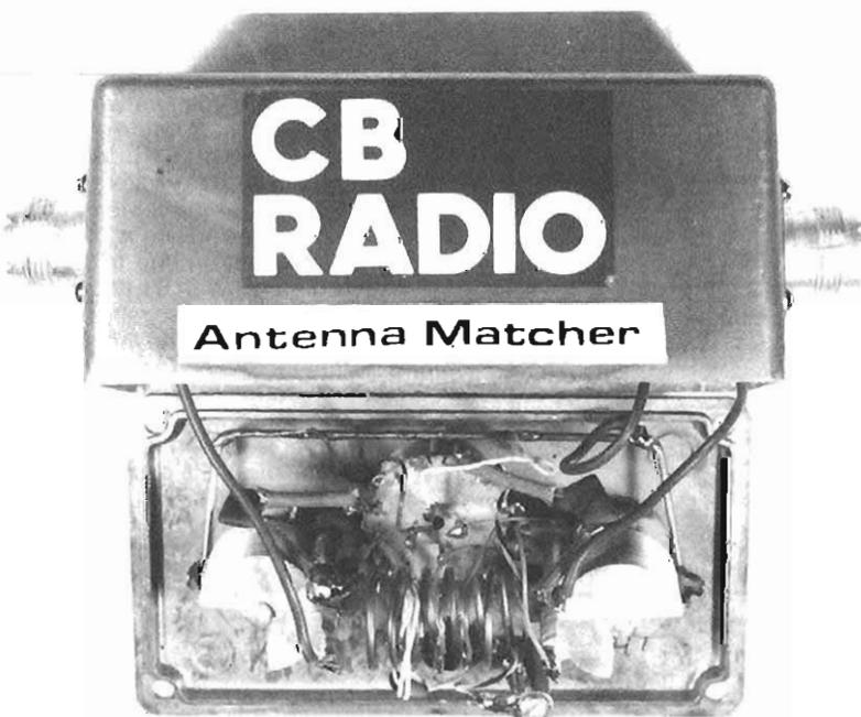
The complete unit showing internal wiring.
