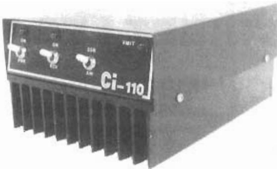
A Solid State, all modes unit covering 1.7 to 38 MHz. Typical power output 130 watts for 215 watts DC input and 4-7 watts drive (15 watts SSB). RF sensing VOX circuit. Switchable receive pre-amp. Supply requirements: 13.8V at 20A, Negative Earth. Size 5" w x 7" l x 3" h. Weight: 2.5lbs.
