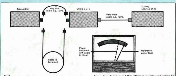
Method of checking the power loss in a length of cable. First set meter to read TX output power with very short cable to VSWR meter. Note reading.
