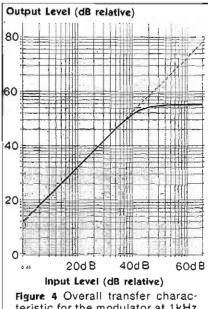
teristic for the modulator at 1kHz
