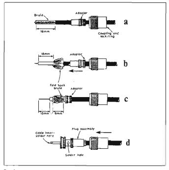
Fig. 3 Cannecting a PL259 co-oxial plug to a small diameter cable. (a and b) Preparation of cable. (c) Fitting adaptor if used. (d) Final connection to alug body.
