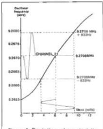
Figure 3 Deviation characteristic for the frequency modulator
