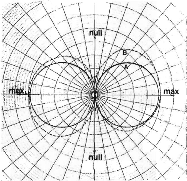
Fig. 1. Polar response pattern of the radio direction finding antenna described in last month's issue of CB Radio Magazine, Radio Direction Finding on 27MHz (Part 2).
