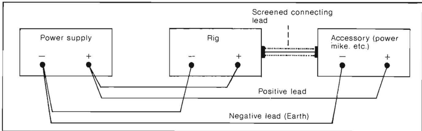
Fig. 1. Showing normal method of connecting on accessory.
