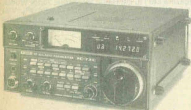
This HF transceiver has a memory which can be recalled, even when on a different band to the one in use and covers from 100kHz to 30MHz. Its cost is justified by such features as an automatic antenna tuner unit, provision for AM, SSB, CW (Morse) and RTTY and needs no tuning or loading. The Icom 720 costs £883.
