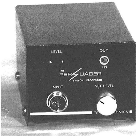
By removing power wasting peaks from the speech waveform and unwanted frequencies the average 'talk power' can be increased by up to THIRTY TWO times, i.e. a ten watt transmitter using the 'PERSUADER' will provide average 'talk power' equal to a 320 Watt transmitter with normal modulation.
