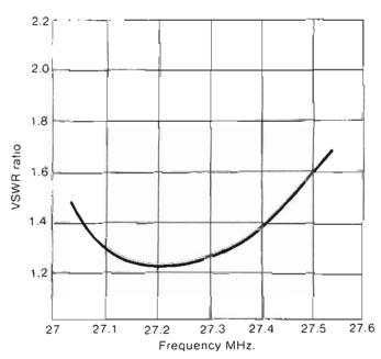
Fig. 1: A typical VSWR curve for the CB band 27 to 27.5 MHz. Minimum VSWR will normally be at approximately band centre but will rise at each end.
