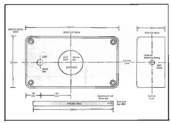
Fig.3: Details for holes in box.
