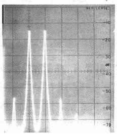
Increasing the input by only 5d8, note the rapid increase in the level of Intermodulation, now at around -42dB. Also note extra signals being generated.
