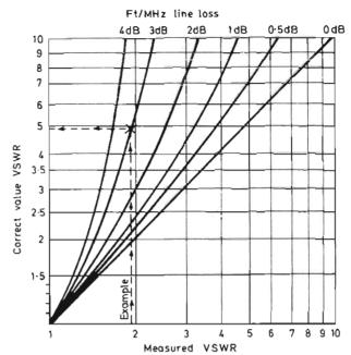
Fig 3: Correction to be made to a VSWR reading to compensate for cable loss. Example: Measured VSWR is 2 to 1 with a normal cable loss of 3dB. The real VSWR is 5 to 1.
