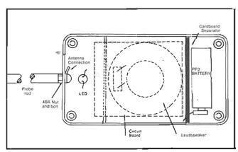
Fig.4: Assembly detail. Circuit board is above loudspeaker.
