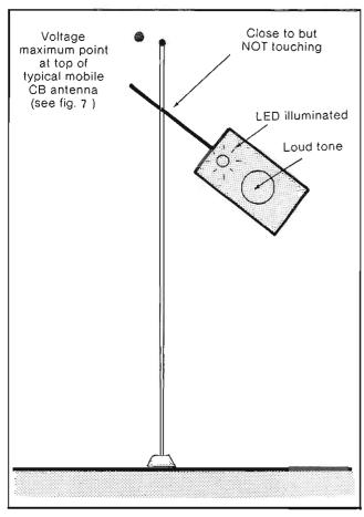
Fig.6: How the antenna checker is operated near an antenna (see text).
