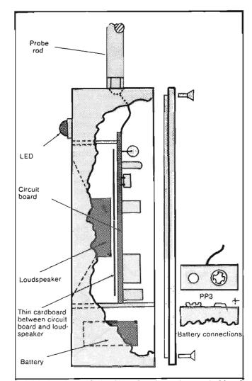
Rig.5: Side view of assembly. Note thin cardboard spacer between circuit board and loudspeaker body.
