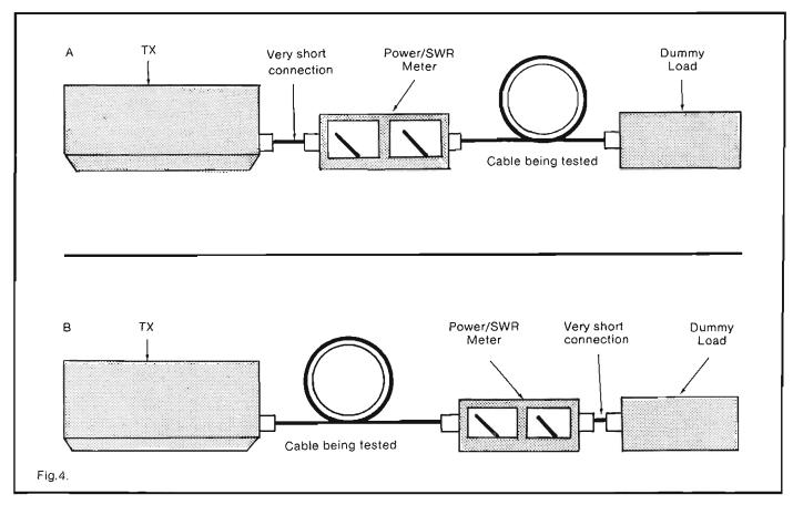
Flg 4: How to check a length of cable for power loss. First measure power going into cable with Dummy Load or end of cable. Then measure power at end of cable going into Dummy Load. With say 10 watts going in and 9 watts coming out the loss is 1 watt or just under 0.5dB (see text).
