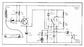
Fig. 1: Theoretical circuit of the antenno checker.
