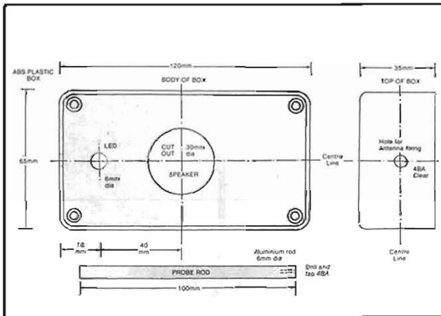
Fig.3: Details for holes in box.
