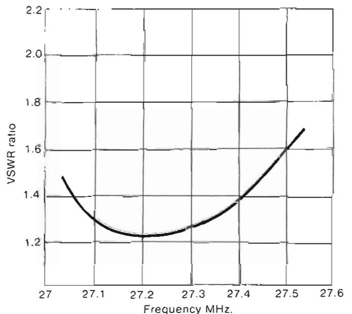
Fig.1: A typical VSWR curve for the CB band 27 to 27.5 MHz. Minimum VSWR will normally be at approximately band centre but will rise at each end.
