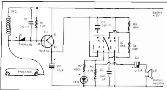
Fig. 1: Theoretical circuit of the antenna checker.
