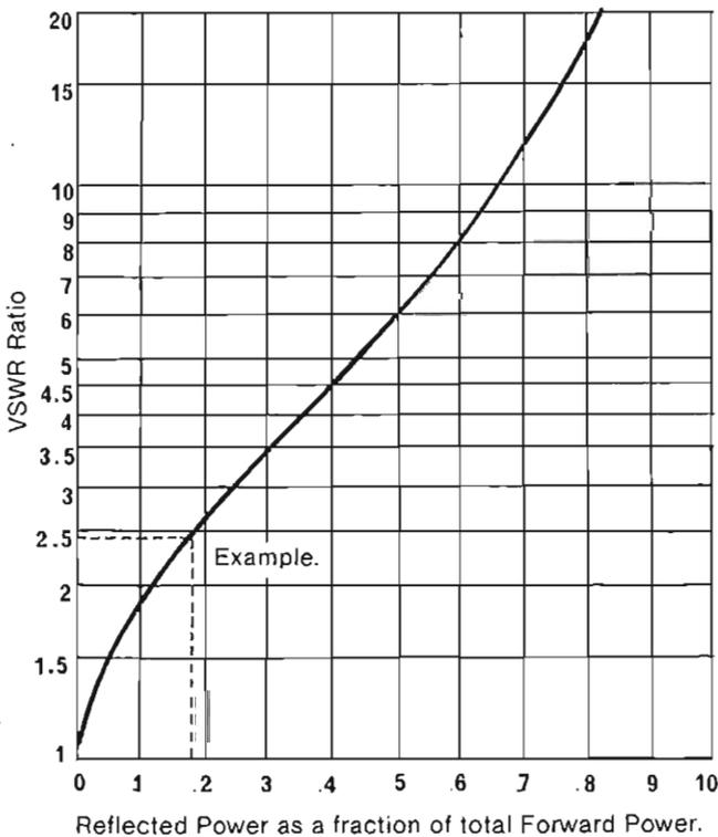
Fig 2: Reflected power and VSWR. The example shows that for a VSWR of 2.5 to 1 the reflected power due to mismatch is nearly 2 tenths of the total forward power. This means that if the transmitter power is 20 watts then 4 watts of that power is returned from the antenna if the VSWR is 2.5 to 1.
