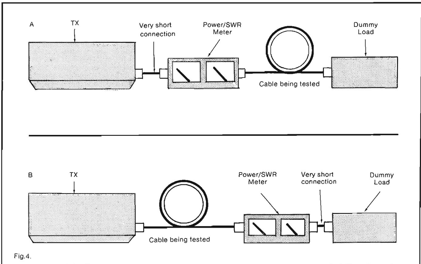
Fig.4: How to check a length of cable for power loss. First measure power going into cable with Dummy Load or end of cable. Then measure power at end of cable going into Dummy Load. With say 10 watts going in and 9 watts coming out the loss is 1 watt or just under 0.5dB (see text).
