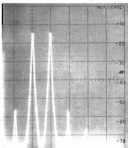
Increasing the input by only 5dB, note the rapid increase in the level of intermodulation, now at around -42dB. Also note extra signals being generated.
