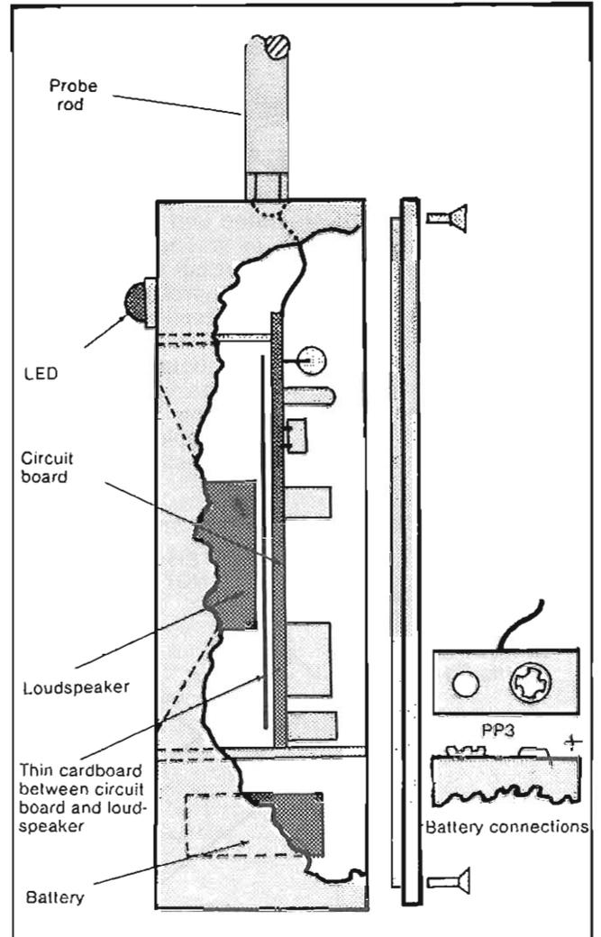
Fig.5: Side view of assembly. Note thin cardboard spacer between circuit board and loudspeaker body.
