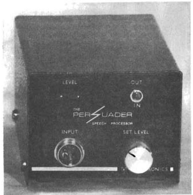
An example of a commercial speech processor which connects between the existing microphone and transmitter input. Units of this type can give considerable gains in average power output without causing the rig to suffer from 'flat topping'. See text.
