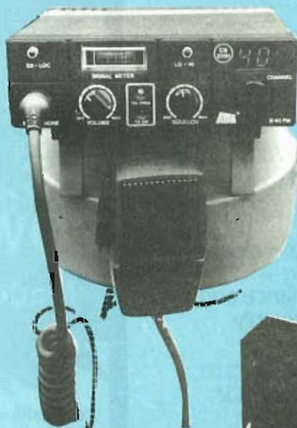
Above the B-40FM with built in mains power supply and hinging legs this is the ideal answer to base station operation
