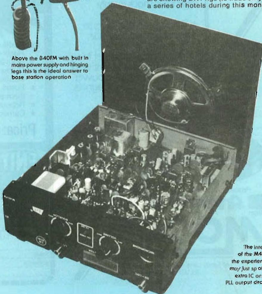
The interior of the M40FM the experienced may just sp of the extra IC on the PLL output circuitry
