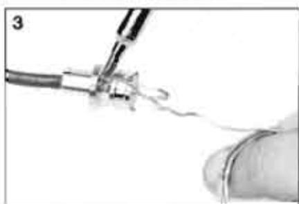
Solder the inner cable to the outer end of the connector. Follow this by soldering the braid to the body of the connector working through the solder holes.
