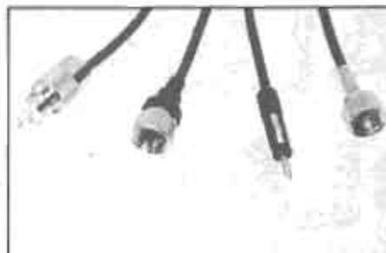
These connectors are less than ideal for connecting the antenna co-axial cable to the c.b. transceiver but still commonly used.
