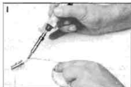
Tin the end of the connector body and braid solder holes to ensure a good electrical joint.
