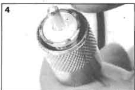
Remove surplus solder from the outer end otherwise it will not slide correctly into the matching connector.
