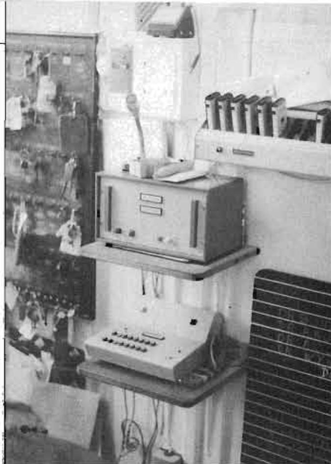
Hospital paging control. Lower unit selects individual bleeper by keying in required identity number. Upper unit sends all numbers for beepers in cardiac arrest team. (Note tulp mike for transmitting location and type of emergency.) Spare beepers for off duty staff are stored above being trickle charged.
