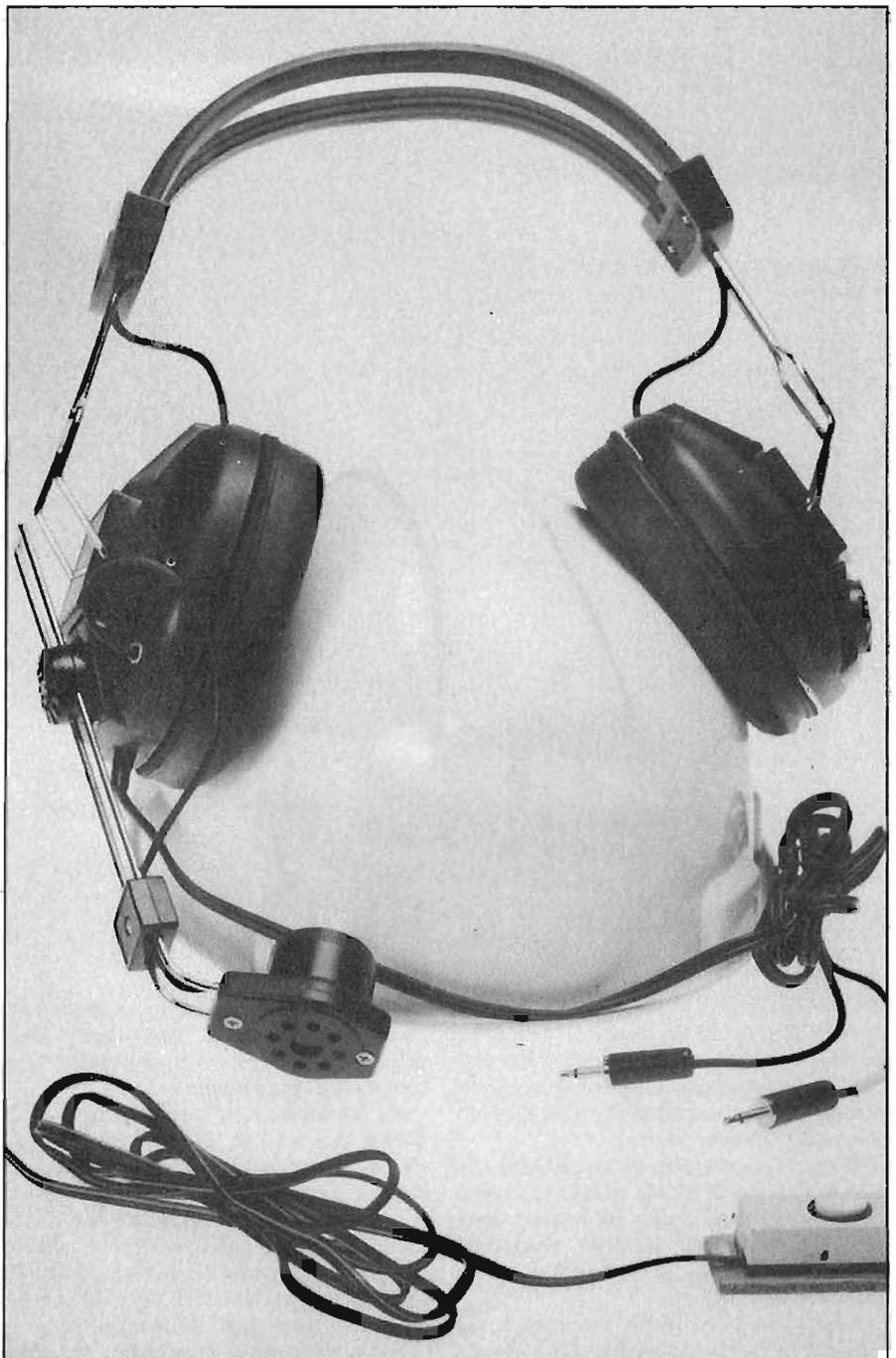
The disabled with home bases can use a pair of headphones. Note the "bell push" switch which can be substituted for the more conventional mike switch. In a car this could be mounted on a tiller control or operated by a foot.
