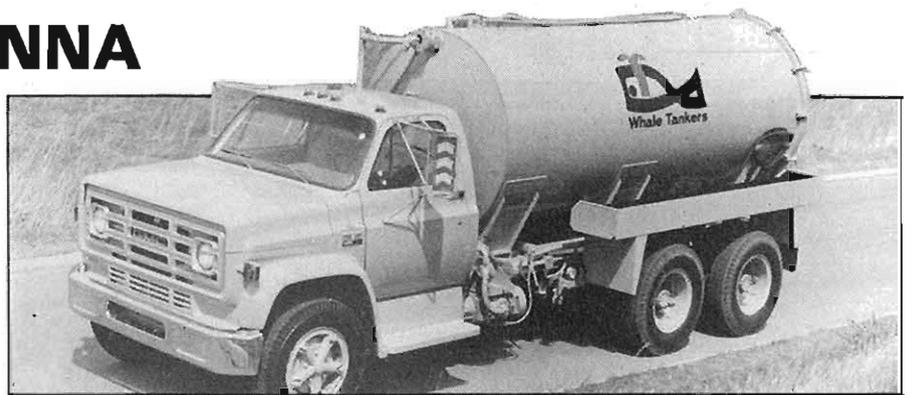
So where would you put the antenna on this vehicle? Remember various ground plane heights can cause SWR adjustment problems as well as giving an unsymmetrical radiation pattern.
