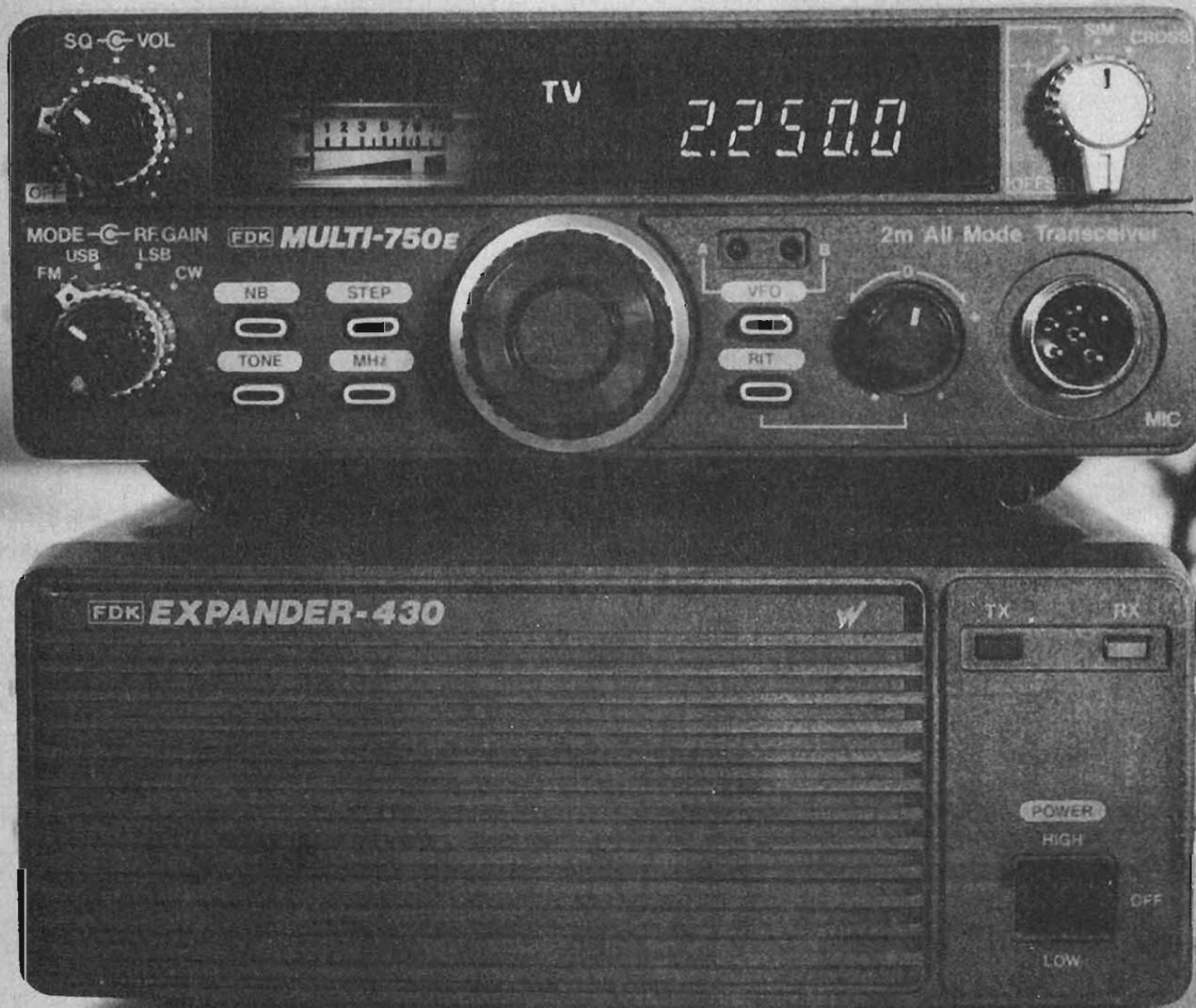
Another mobile or base station with a UHF adaptor. The transceiver features 10 watts on FM/SSB/CW 144-146MHz. The adaptor gives operation in the UHF band 430-440MHz by a press of a button.
