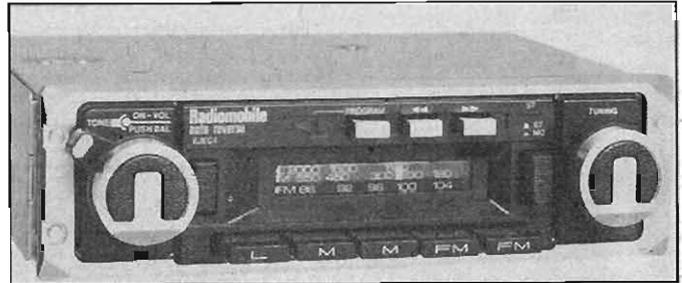
The Radiomobile 536 combined auto reverse car stereo cassette player and radio covering L, M, and FM wavebands.
