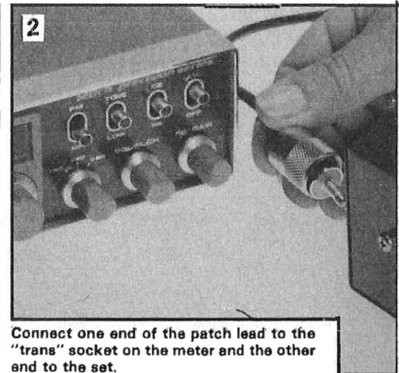
Connect one end of the patch lead to the "trans" socket on the meter and the other end to the set.
