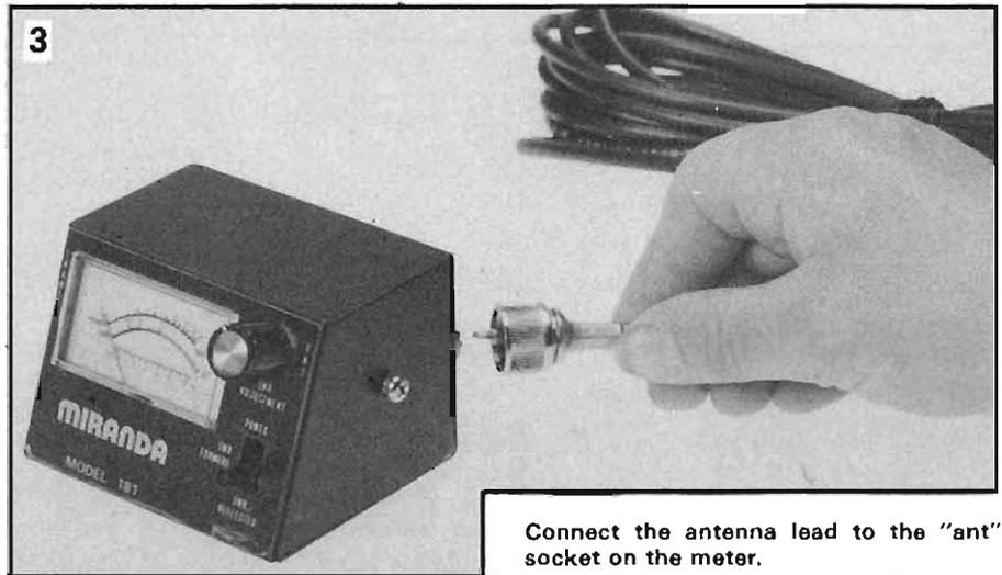
Connect the antenna lead to the "ant" socket on the meter.
