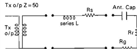
**Complete theoretical circuit of proposed antenna. The antenna is assumed to have a length of 1.5 metres and a diameter of 6mm.**
