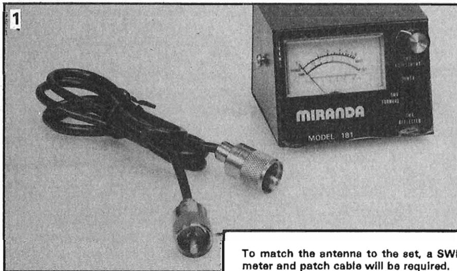
To match the antenna to the set, a SWR meter and patch cable will be required.
