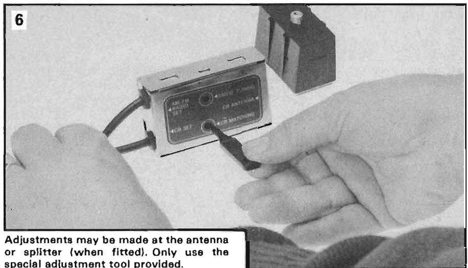
Adjustments may be made at the antenna or splitter (when fitted). Only use the special adjustment tool provided.
