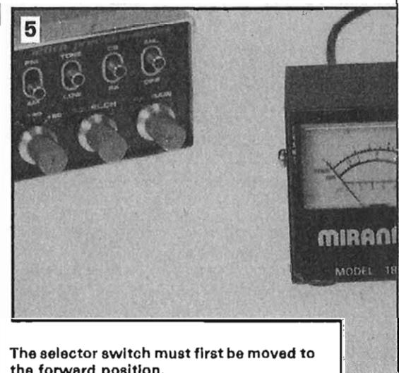
The selector switch must first be moved to the forward position.
