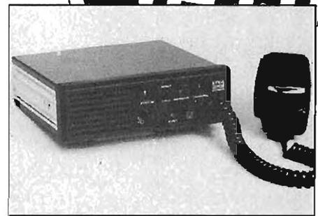
The M2010AM/SD1 radio telephone from the Dymar Lynx series. It's 7½ watt, 10 channel between 148 to 174 MHz. Er . . . it's also double-sideband a.m. But Dymar won't make c.b.
