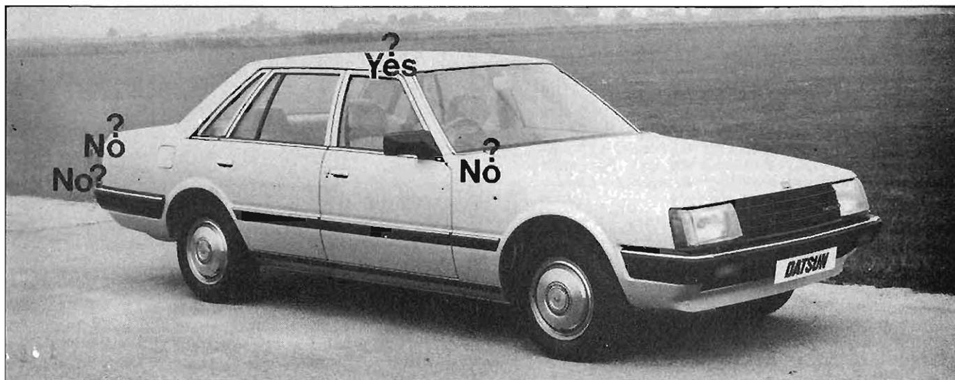
The centre of a vehicle's roof is the best location for the antenna.
