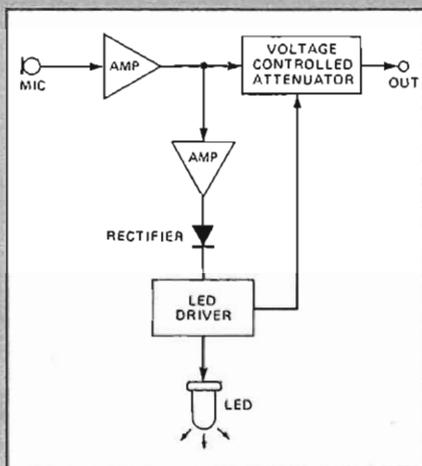
ator and a fixed attenuator. The gain of the amplifier is balanced by losses through the attenuator so that the unit has unity gain overall. Pre-amplification is necessary to provide a high signal level to the VCA input, so that unwanted switching pulses generated by the circuit are small in comparison to the speech signal. The attenuator then restores the signal to its original level.
