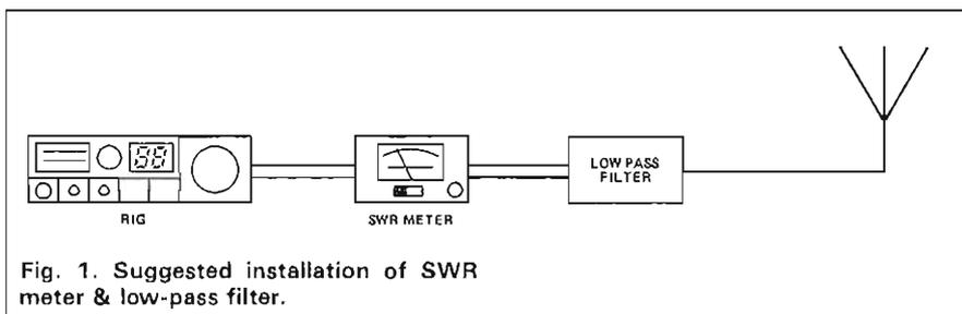
Fig. 1. Suggested installation of SWR meter & low-pass filter.
