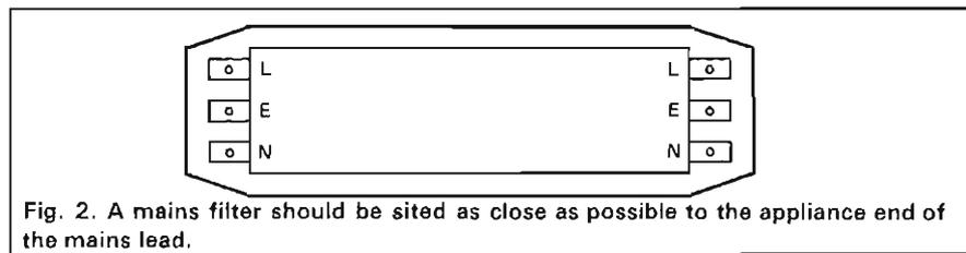
Fig. 2. A mains filter should be sited as close as possible to the appliance end of the mains lead.
