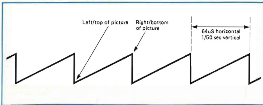
Figure 3. Timebase waveform
