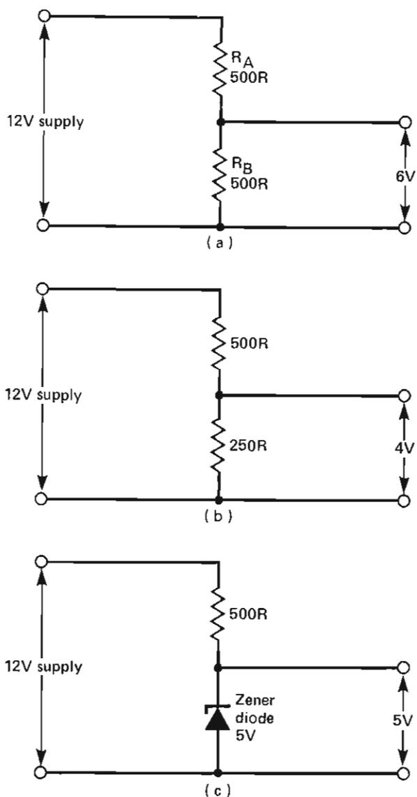
Figure 5. Potential dividers and the zener diode
