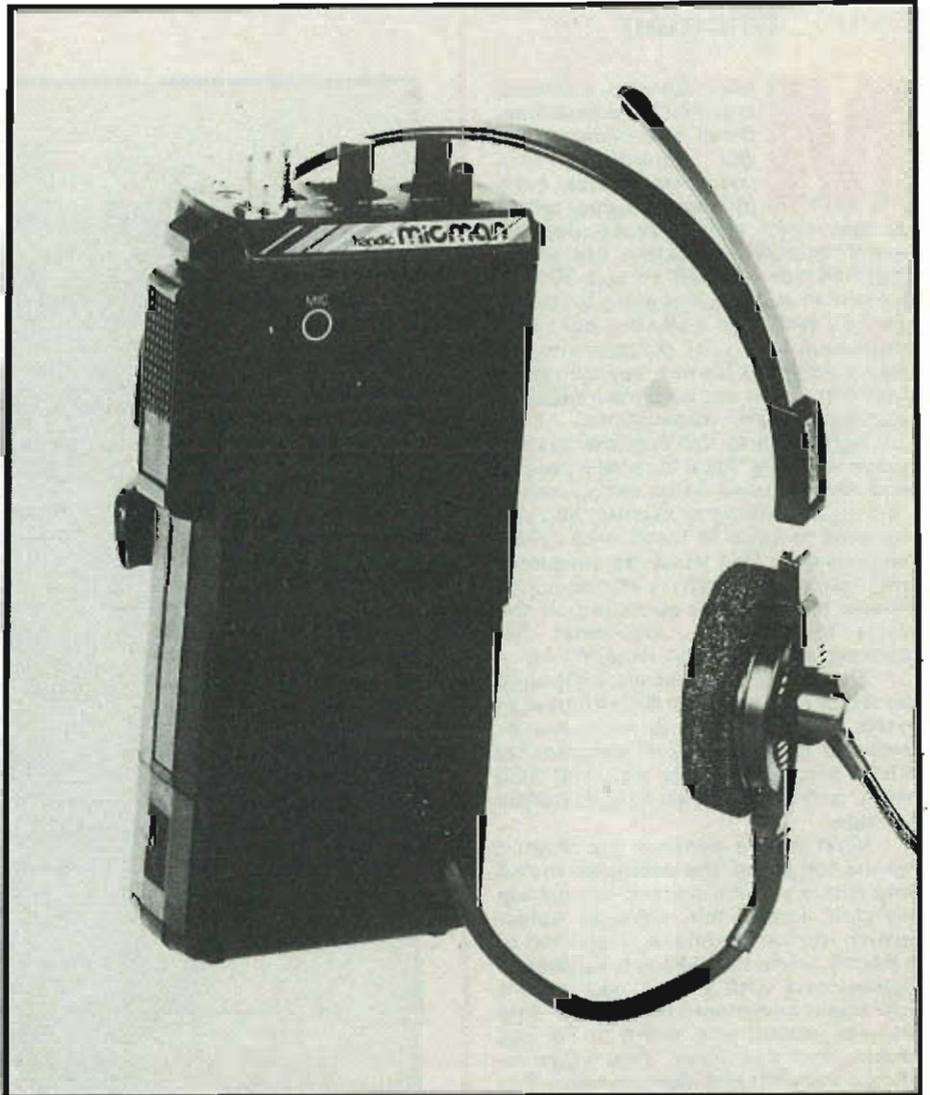
This facility would lend itself to other applications, and it would be possible to have a base station and use the units as a pager with answering possibility. Up to 12 handhelds can be called from, for example, the switch-board of a company, or used on a farm.
