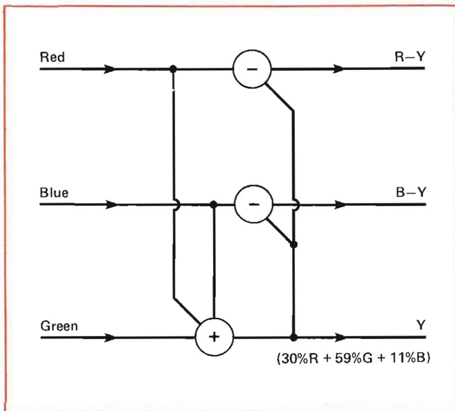
Figure 7. Obtaining colour-difference signals
