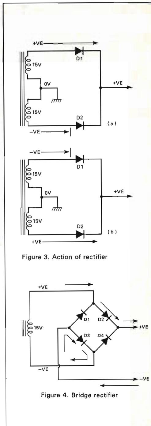
Figure 3. Action of rectifier
