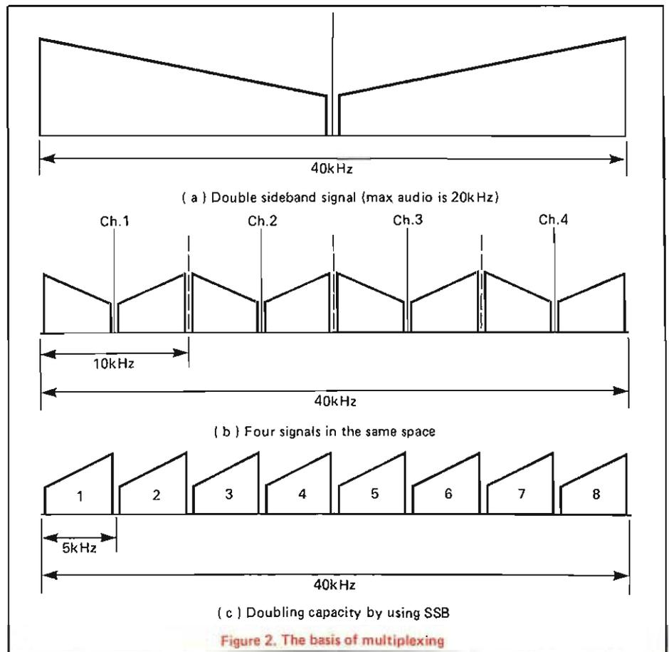
Figure 2. The basis of multiplexing
