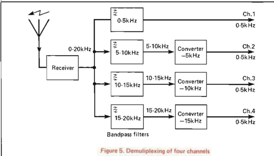
Figure 5. Demultiplexing of four channels
