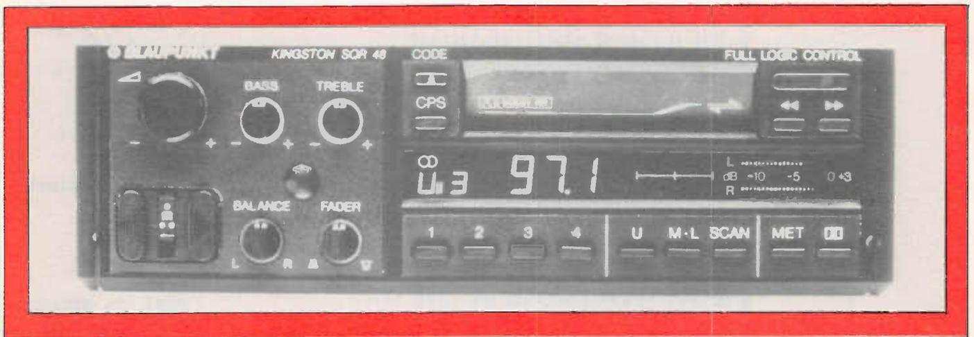
the market. It, too, has a three-waveband Codem III PLL tuner with manual and automatic up/down scan, FM auto-scan and a 20-preset station memory. All that's missing is the preset scan. The tape section has the same logic-programmed soft-touch controls, auto-reverse, programme search and Dolby B noise reduction.
