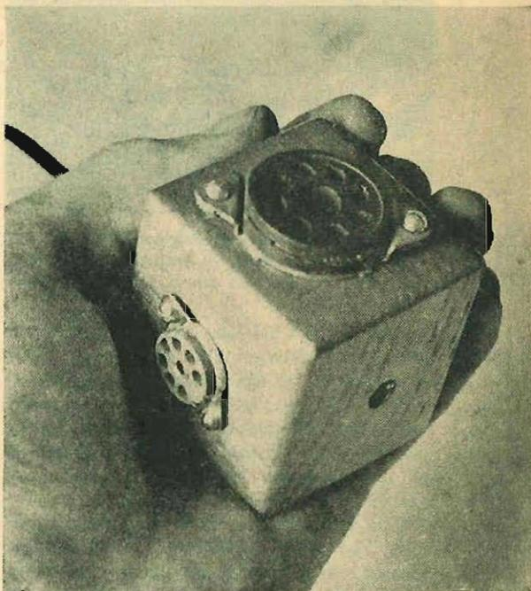
Made from a single piece of 2 x 2-in. stock, CB Cube Tester checks most tubes for open filaments.
