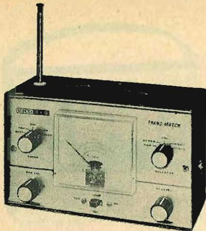
EICO's 715 Test Set is designed to ring out the entire C.B. transceiver—it's self-powered.
