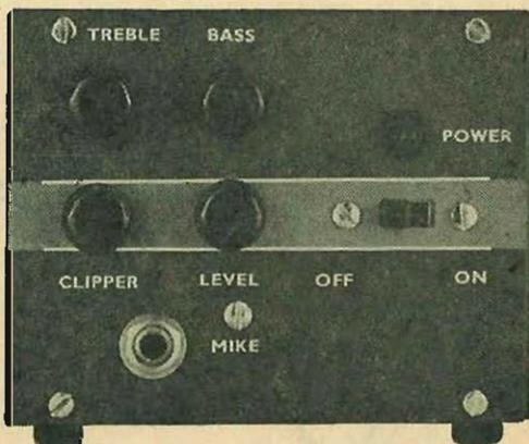
on front panel (right) could be screwdriver adjustments or locking-type potentiometers since none of the controls are varied constantly—once set they need not be changed again.
