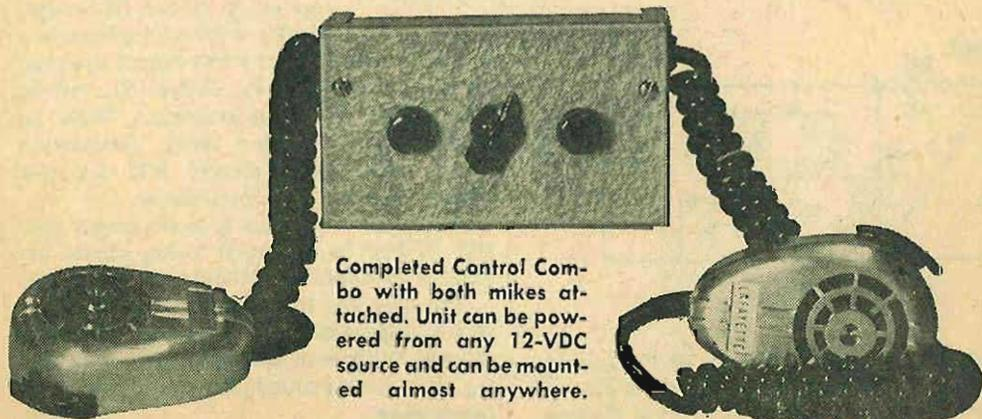
Completed Control Combo with both mikes attached. Unit can be powered from any 12-VDC source and can be mounted almost anywhere.
