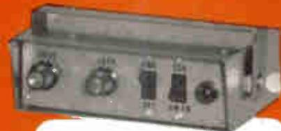
CONTEX model 7001 is one of the worlds smallest mobile linears (only 6"x6"x2"). It's all solid state - which means it draws only 100 milliamps in standby, and approximately only 5 amps in transmit. Up to 40 watts RF output ..... \$139
