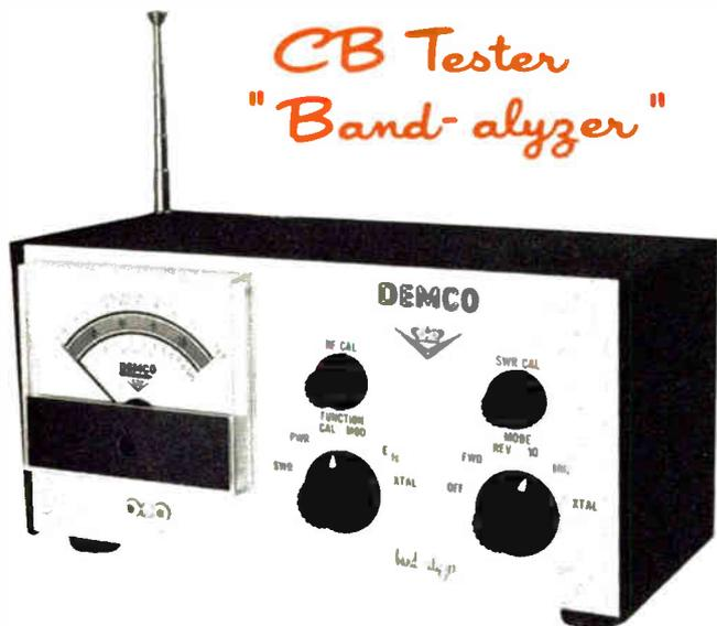
DEMCO "Band-alyzer" CB Tester lets you know how your unit is functioning. Usable on base or mobile. Measures standing wave ratio, measures power output to 1000 watts, indicates modulation percentage, measures relative field strength and checks crystal activity. Size: W 6" X H 4-1/2" X D 5-1/4". . . . . \$59.95
