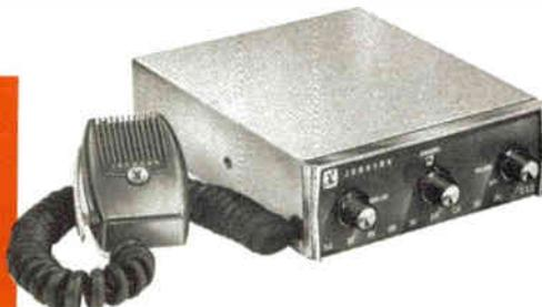
**JOHNSON MESSENGER III** is a 12vdc, 12-channel Solid State CB transceiver. Dual conversion means a better receiver. Multi-stage automatic noise limiter. Noise immune squelch. Illuminated channel selector. Paging feature. External speaker jack. Provisions for tone alert. 2½" h, 6¾" w, 8¾" d. Supplied with crystals for channel 9, microphone, and mobile mounting bracket . . . . . **\$149.95**
