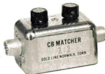
**GOLD LINE GLC-1046** Antenna Matching Network stops power loss due to high SWR. A perfect SWR is 1.1 to 1. If your SWR is 1.5 to 1 you're losing up to 20% of your transmitting power. If your SWR is 2.1 you're losing 30% of your power. Simply insert the GLC-1046 Antenna Matching Network between the transmitter and the antenna lead-in with a SWR meter and tune for minimum SWR.....\$9.98
