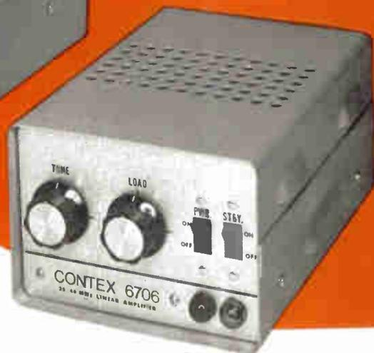
CONTEX Models: 6706 (Base) and 6801 (Mobile) linear amplifiers provide up to 80 watts output. (18db power gain) Uses a pair of 6JG6A tubes in the Final. 6-3/8" w, 4-3/4"h, 9"l
