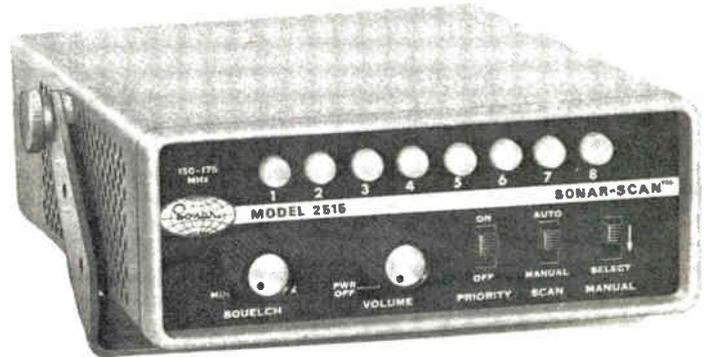
The SONAR AUTO-SCANNER is an FM monitor receiver that will signal-search and automatically lock a signal on any of 8 programmed channels. A Priority Channel signal will lock to the exclusion of all other signals. Carrier Delay allows you to hear mobile callbacks (if on the same channel). Manual selection is accomplished by Slow-Scan technique. 117vac or 12vdc. 7" x 2 1/4" x 8 1/2" Sonar Model FR-2514 for 25-50 MHz FM.....\$189.95
