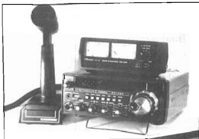
*SSB Yaesu transceiver FT707 with SWR and power meter.*
