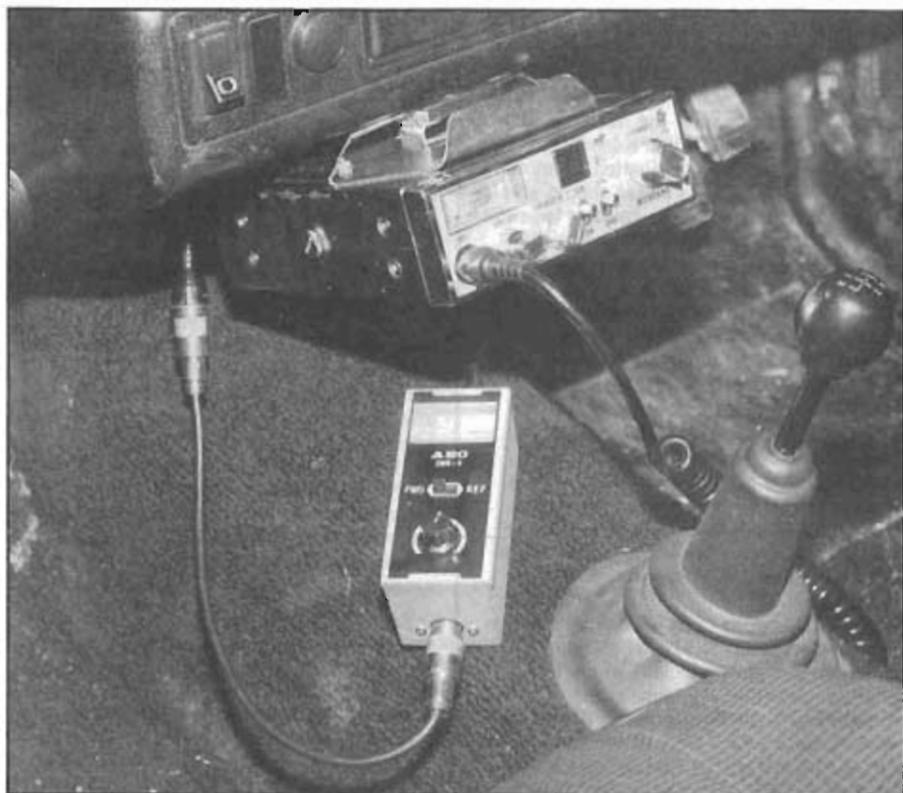
Rig and slide mount in position with SWR meter connected in line ready to give SWR reading.
