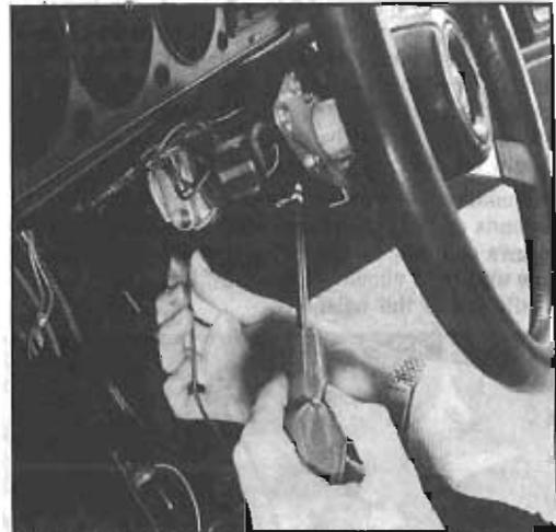
*A good earth is imperative. Here the indicator and flasher switch mounting bracket is being utilised.*
