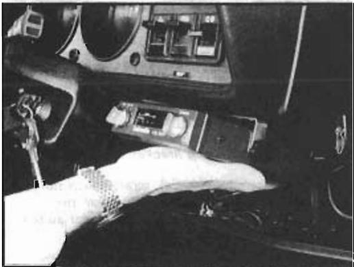
When fitting, make sure the rig is within easy reach, and if there is a window (as in the Radiomobile unit) check that it doesn't reflect the sunlight into your eyes.
