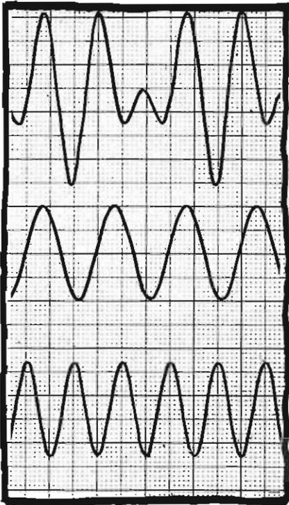
Hidden frequencies! At first glance one does not notice that the upper curve is the sum total of two curves with different frequencies.
