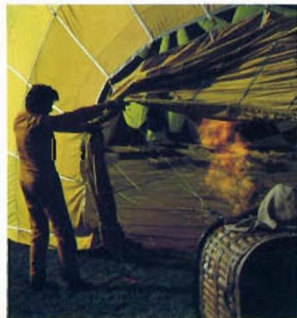
The preparations for the start begin with the heating-up of air in the envelope.
