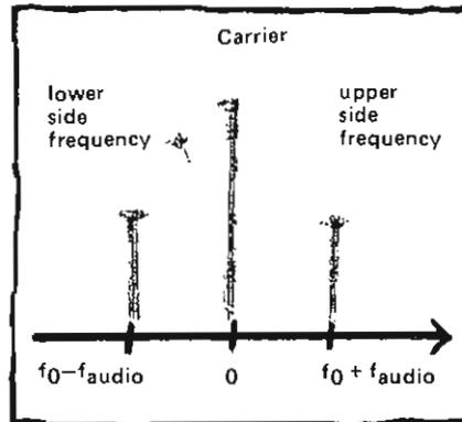
If a carrier oscillation is AM-modulated with a tone, two side frequencies emerge.
