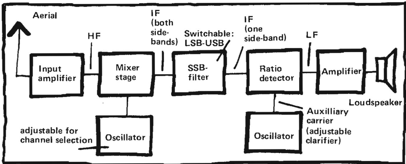
Block diagram of an SSB receiver operating according to the superhet receiver principle. The SSB-filter serves to select the desired
