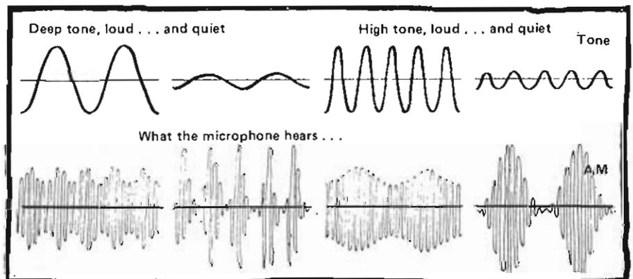
To remember, we have here once more the diagram in which the A, modulation is illustrated. The black curve on top represents the tone vibration. The coloured curve be-
