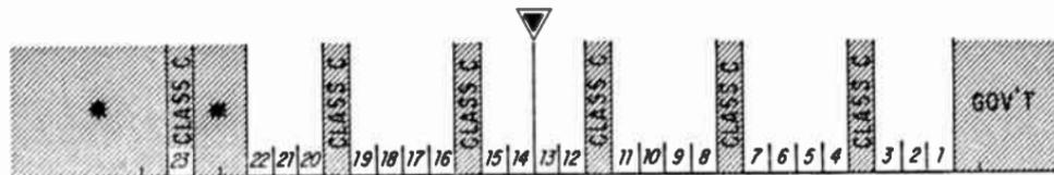
On the left stars indicate channels used by public safety, land transportation, and industrial radio services. The small triangle points out the center frequency used by industrial, scientific, and medical devices. \* On the right are channels used by the government. And in between the CB channels are Citizens' Radio Class C station users.
