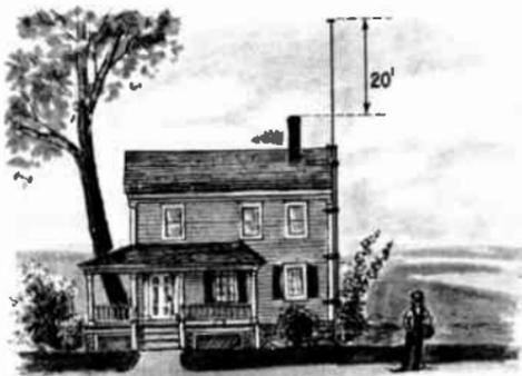
13. You may also mount CB antennas on trees or on the ground. The antenna may not be more than 20 feet above the tree or ground.
