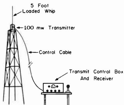
FICTION—Mounting the transmitter at the top of a tower (to eliminate feed-line loss) and using a loaded whip (not longer than 5 feet) has given some users coverage not far behind many of the Class D 5-watt input stations in their area.
