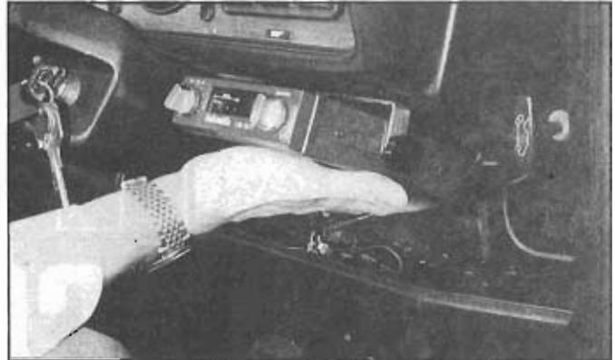
5. Now we come to fit the rig. Decide where the radio is to go, bearing in mind the other components around it, like the bonnet release, your legs, and does it prevent you from using the tray under the dashboard? Offer it up temporarily to make doubly sure.
