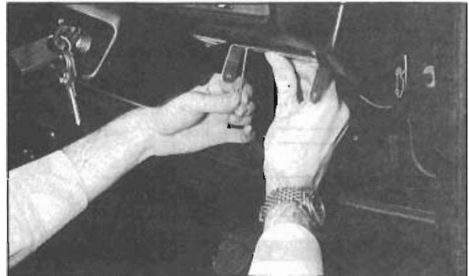
6. Work out where the mounting holes will go. Here we use a drill as the guide. Check there are no wires behind the fascia before you begin to drill the holes. The result here could be a nasty short, blown fuses, and at worst burnt out instruments!
