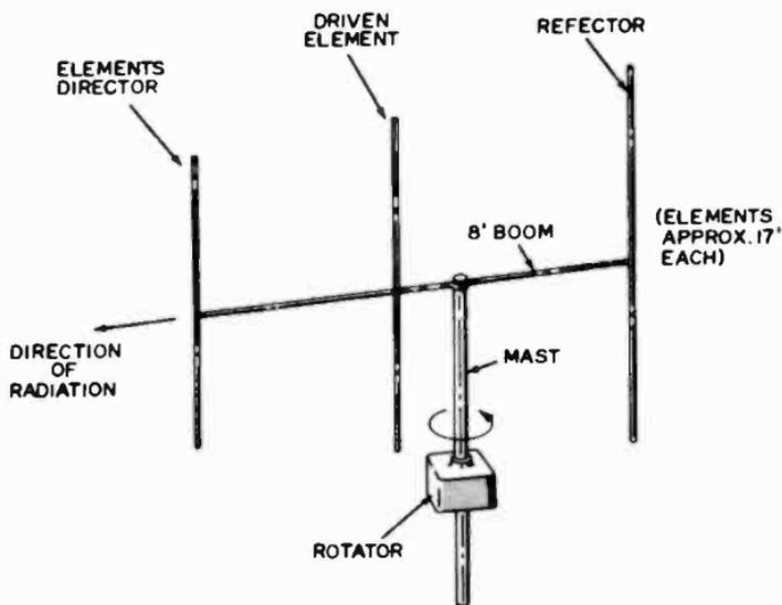
Fig. 5-5. Vertically polarized 3-element directional beam.
