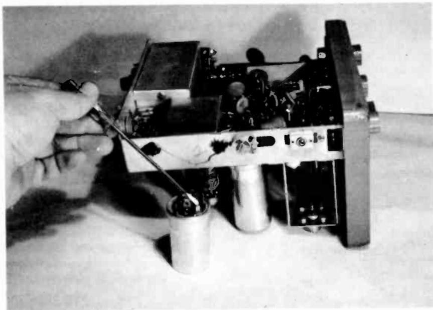
Fig. 9-1. Shorting filter capacitor to prevent shock.
