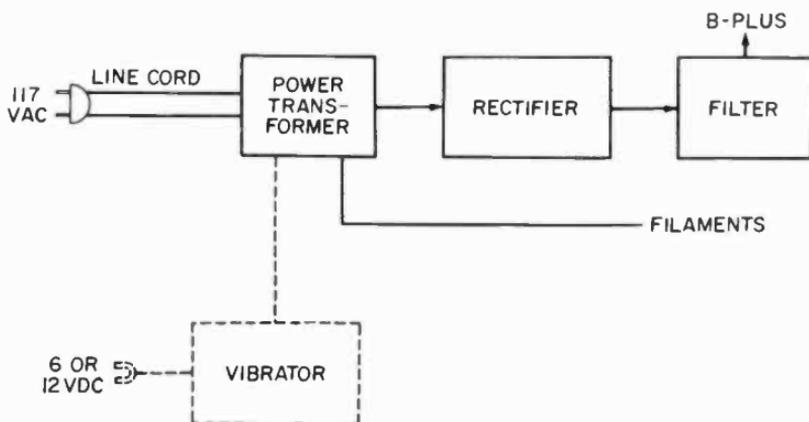
Fig. 4-3. Block diagram of a power supply.
