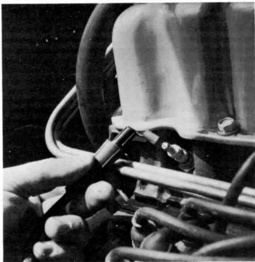
**Fig. 6-2. Spark-plug suppressor clipped between plug and cable.**
