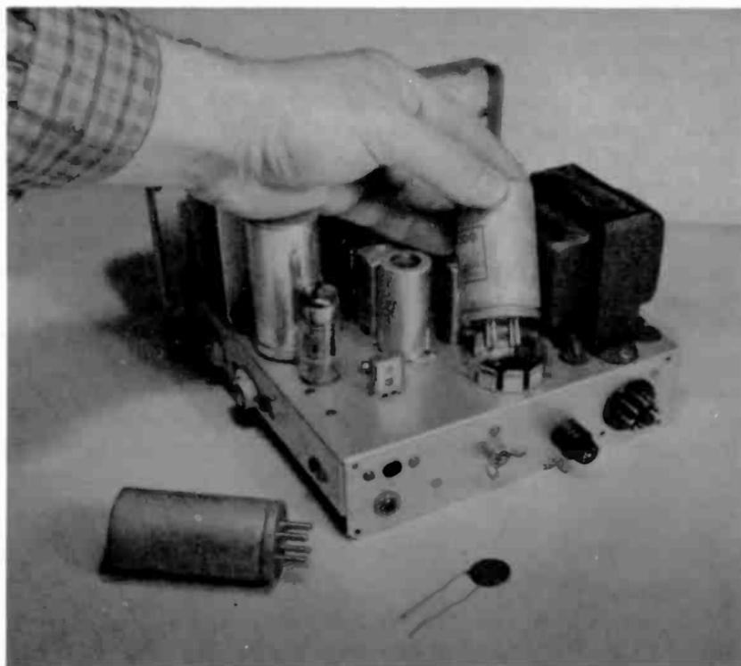
**Fig. 9-5. Replace buffer capacitor when installing new vibrator.**
