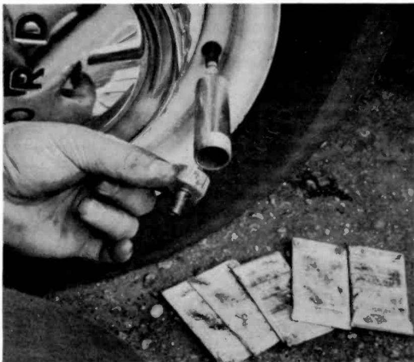
**Fig. 6-6. Special tool and packets of antistatic powder.**
