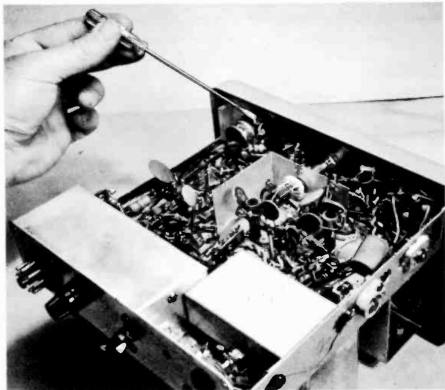
**Fig. 9-6.** Click test with screwdriver tip applied to control lugs.
