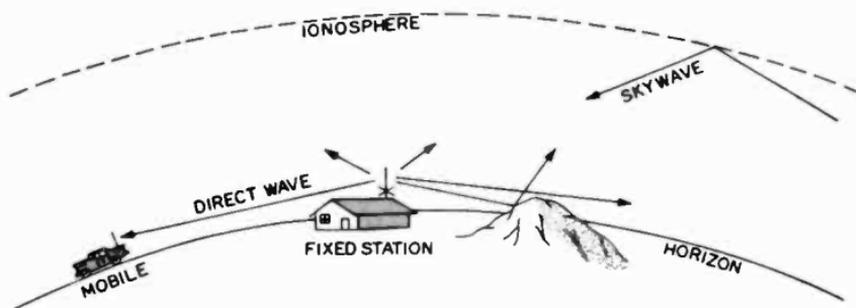
**Fig. 5-1. Behavior of CB radio waves.**
