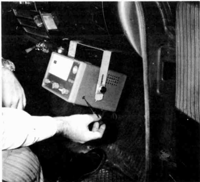
Fig. 7-5. Tuning transmitter of a mounted unit.
