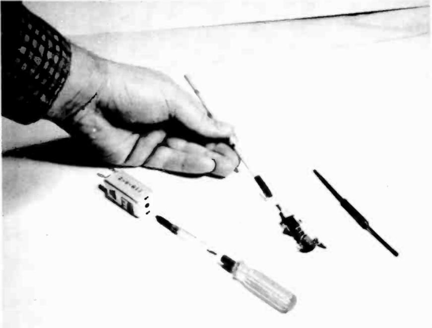
**Fig. 7-1. Alignment tools for CB equipment.**
