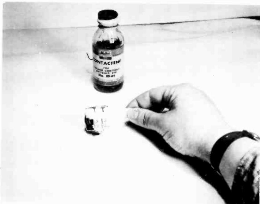
Fig. 9-2. Cleaning send-receive relay contacts.
