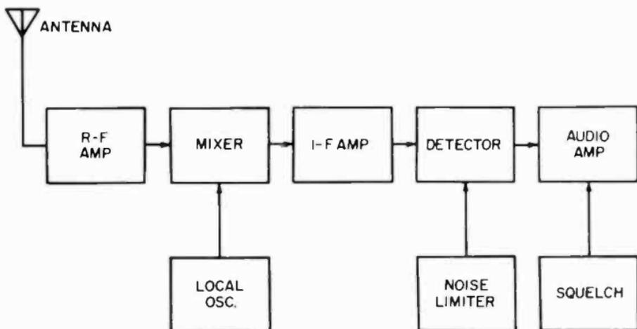
Fig. 4-2. Block diagram of a superheterodyne receiver.
