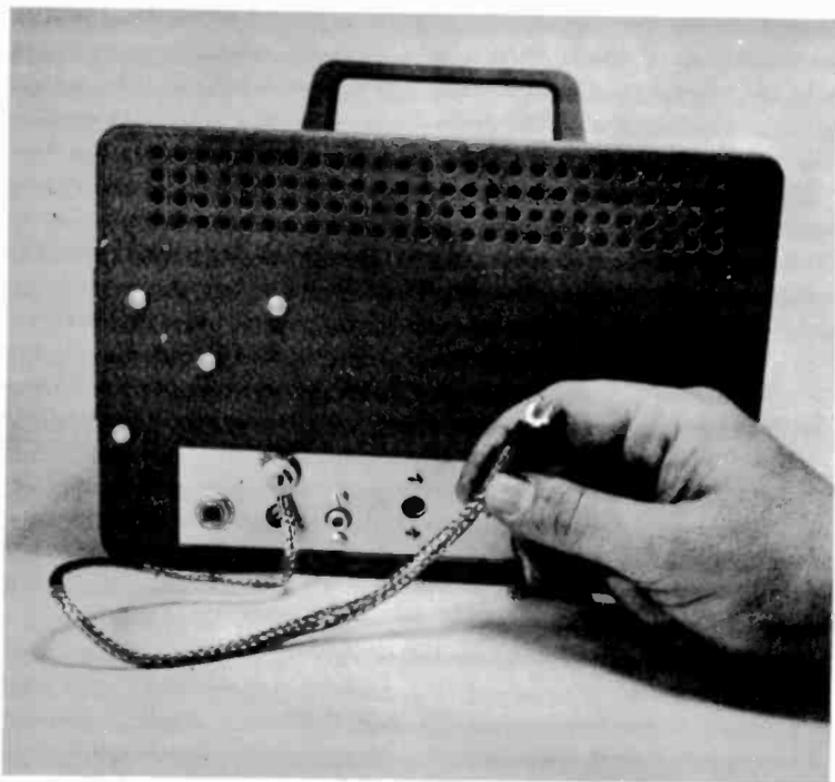
Fig. 6-1. Ground lead connected to transceiver.
