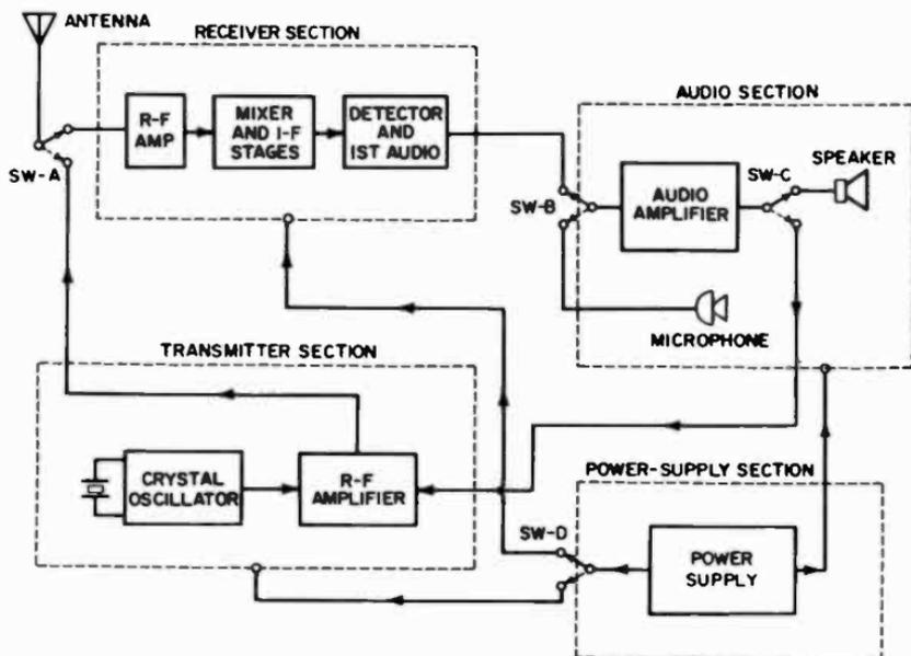
Fig. 4-1. Block diagram of a typical transceiver.
