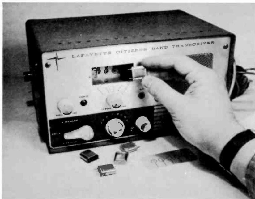
**Fig. 10-3. Exchanging crystals between units of different manufacture might cause off-frequency operation.**
