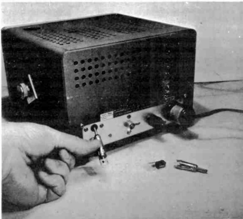
**Fig. 7-2. Dummy load made from #47 pilot lamp and antenna plug.**
