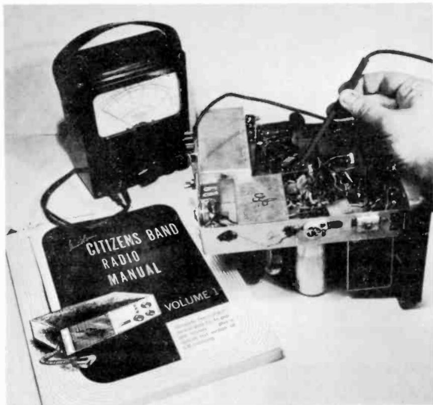
Fig. 9-3. Service literature plus voltage and current measurements will pinpoint most troubles.
