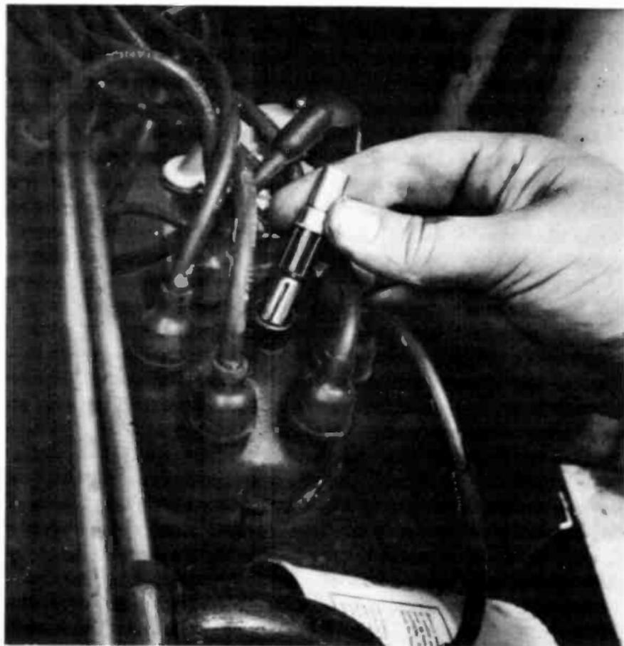
**Fig. 6-3. Installation of distributor suppressor.**
