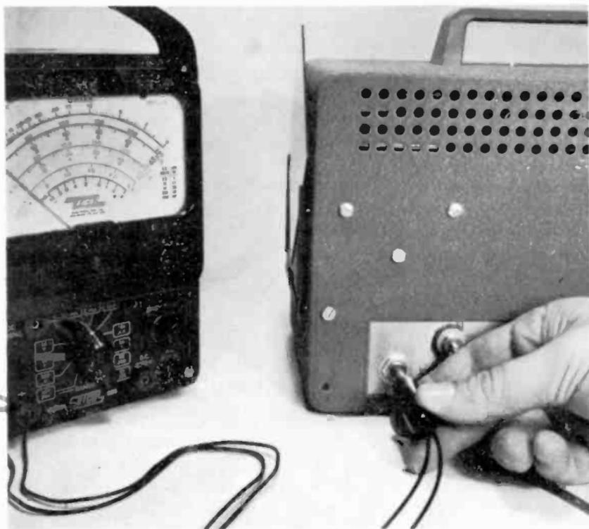
Fig. 7-3. Measuring power input with a multimeter.
