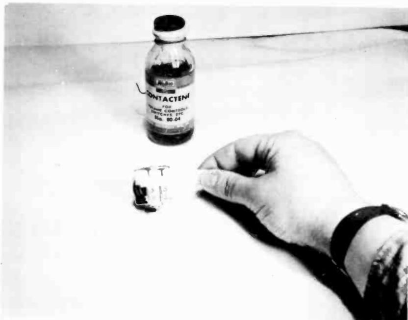
Fig. 9-2. Cleaning send-receive relay contacts.
