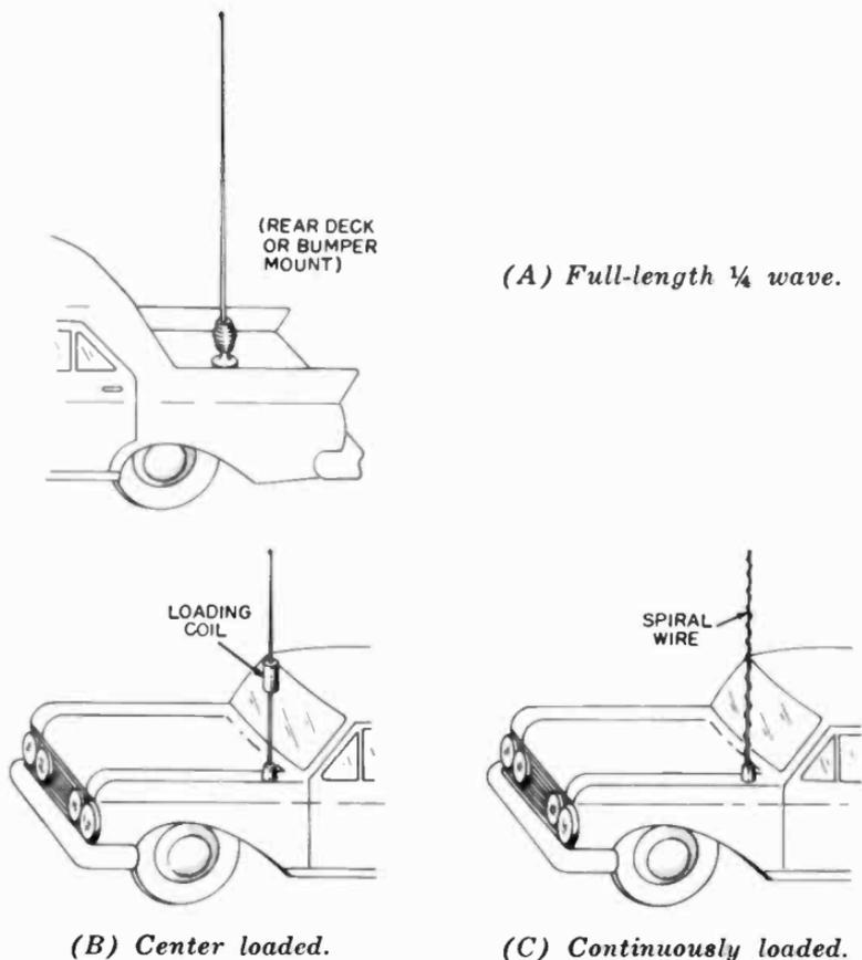
Fig. 5-4. Basic mobile whips.
