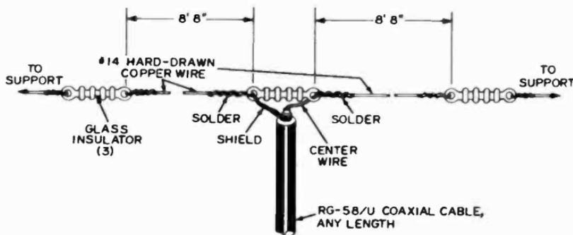
Fig. 5-2. Construction detail of dipole antenna.
