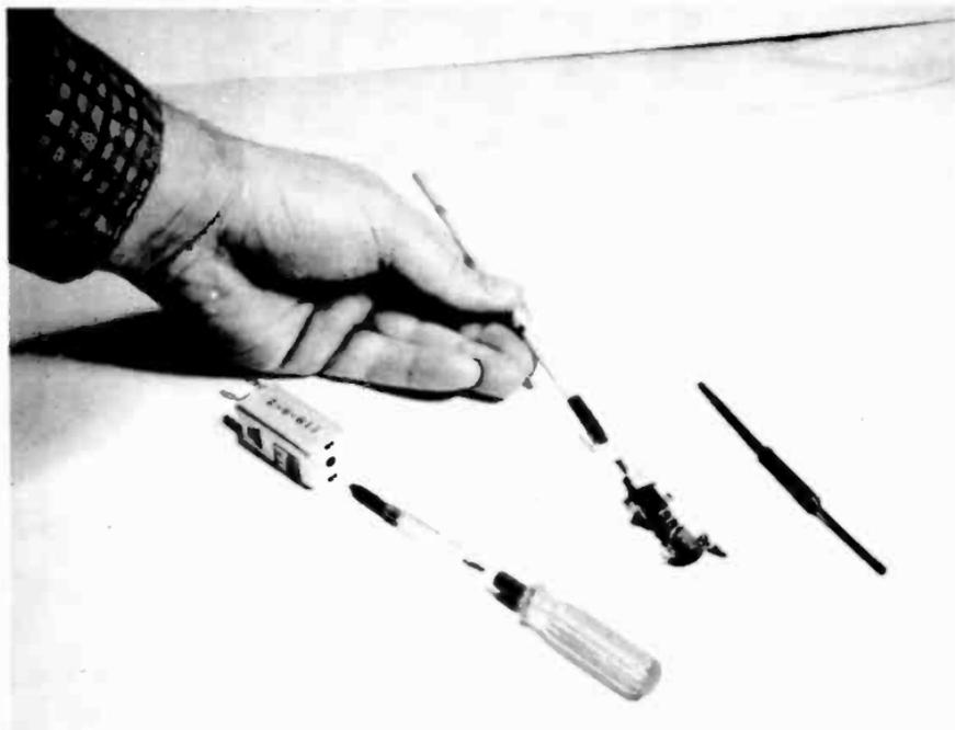
**Fig. 7-1. Alignment tools for CB equipment.**
