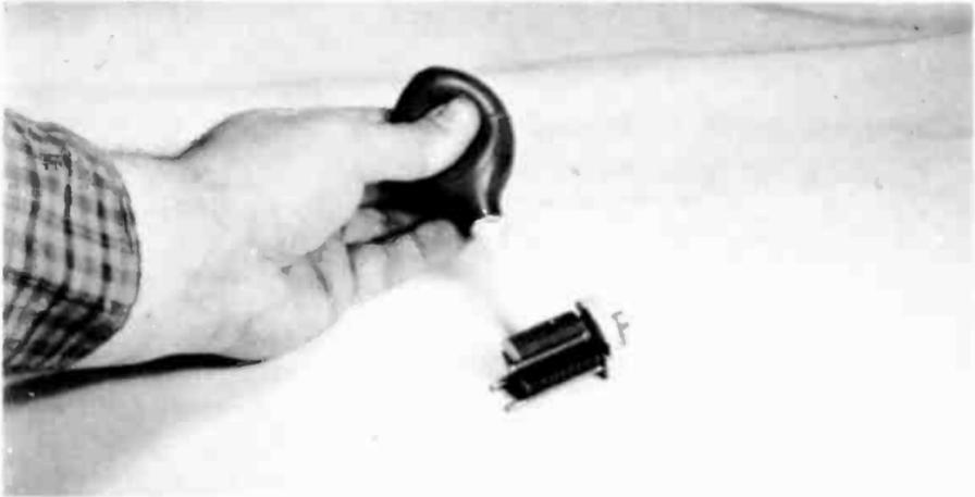
Fig. 9-7. Rubber bulb is useful for blowing out dirt.
