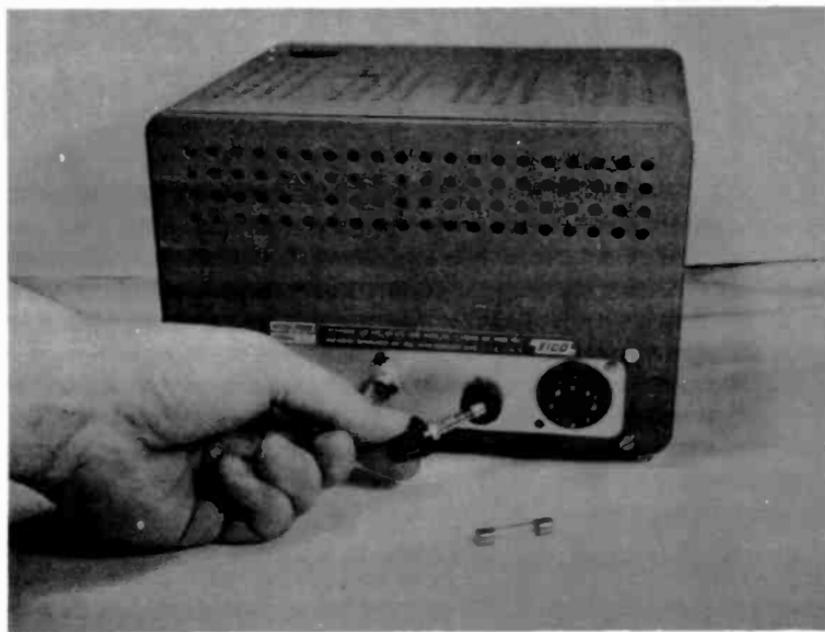
Fig. 9-4. Different fuses are often used for car and home operation.
