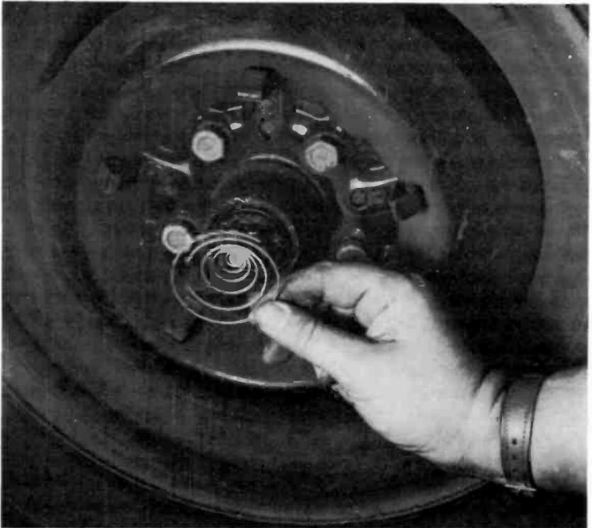
**Fig. 6-5. Static collector springs installed on front wheel.**
