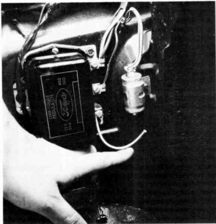
Fig. 6-4. Generator bypass capacitor.
