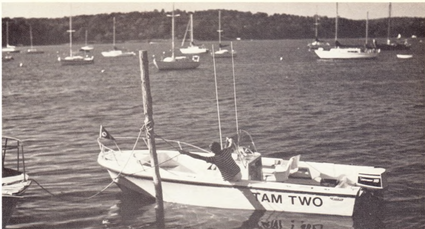
Even small craft have their ears on when they put out from shore. One of the two half-wave marine antennas on this runabout is for CB. Boaters use the name of their vessel as a personal handle.
