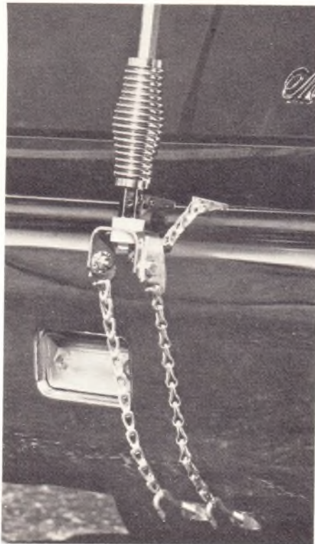
This bumper mount, secured by dual chains, exposes the antenna base to damage by somebody else's bumper.
