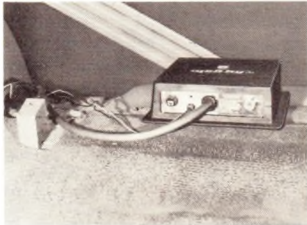
Trunk-mounting Step 3/The closer you mount the transceiver to the rear-seat back, the safer it is from damage.
