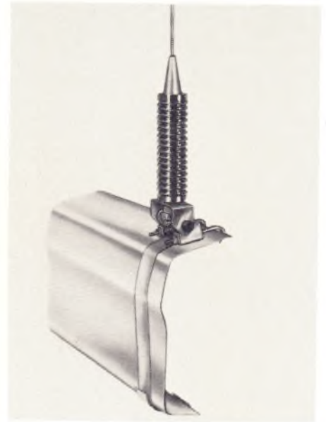
Stainless-steel strap and short adjustable hooks on this Turner bumper mount allow positioning antenna base where it's less vulnerable.
