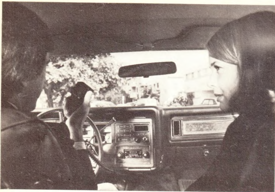
You don't use scarce dashboard real estate with an in-dash mount. This AM/FM/Tape/CB unit by J.I.L. blends with the vehicle's interior trim.
