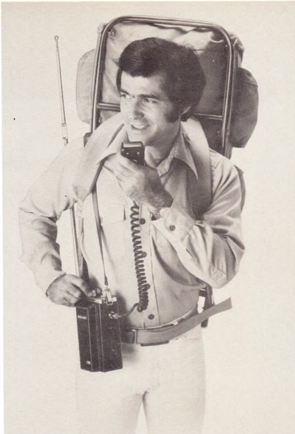
This footloose CBer is operating his Midland 13-861 on rechargeable batteries. When he hikes back to his car, he can operate mobile from the vehicle's electrical system.
