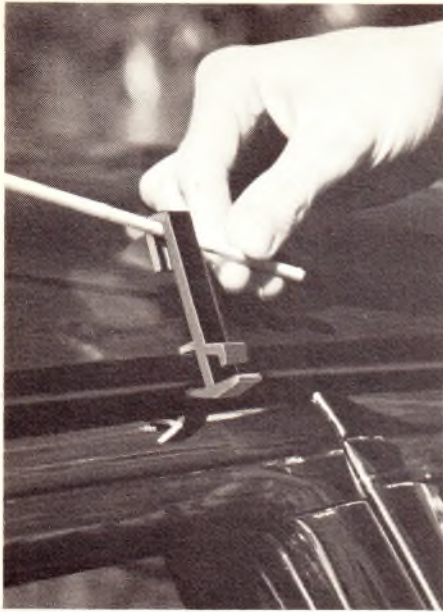
Clip your whip. Accessory clips fasten the antenna tip to the rain gutter so you can garage your vehicle.
