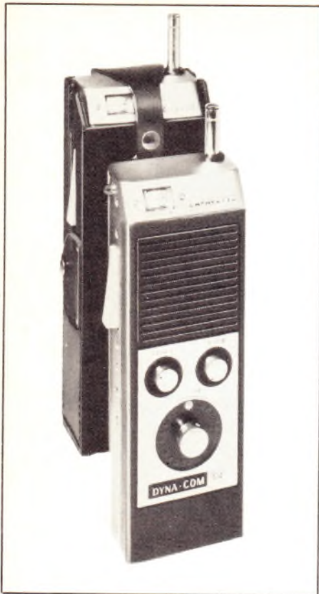
Portable sets should be protected from dirt and moisture which can enter through exposed plug-in connectors on set. This Lafayette Dynacom 23 has a flap which closes over the connectors for protection.
