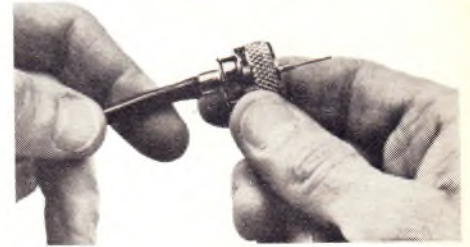
Slide the coupling nut over the connector body. Hold cable in one hand and use other hand to push ferrule over barb until braid is captured between ferrule and connector-body flange.
