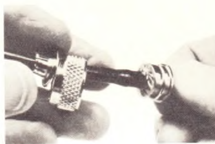
When body assembly is properly positioned, the braid fans out against rear flange or body.
