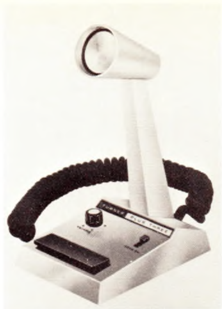
Add a power mike with speech compression for improved modulation. This Turner Plus-3 has battery-powered mike amp in base; the black bar is a press-to-talk switch that can be locked on for convenience.
