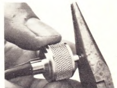
Squeeze-crimp the tip of the center contact.
