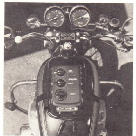
Motorcycle mounting Step 6/With this Beltek Enduro 23, 2-wheelers have the same CB benefits that 4- and 18-wheelers enjoy. After mounting the antenna, secure cable under or along the lower edge of seat.
