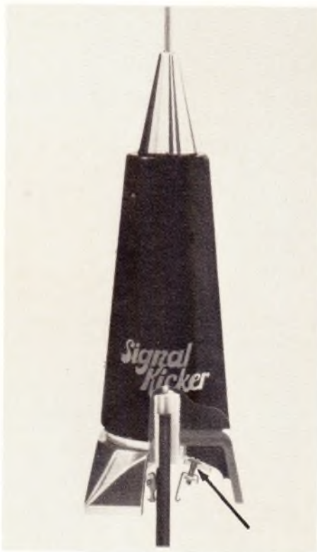
This roof-mount installs entirely from the outside. Drill hole, position mount, tighten screws (arrow) which pull claws against roof metal.
