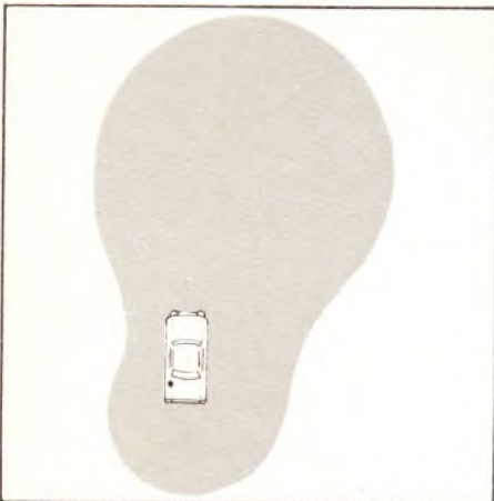
Cowl mounting puts more signal where you've been. Rear fender mounting gives you a bit more range to where you are going. Both patterns are slightly angled by off-center antenna.
