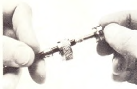
Push barbed barrel of connector body so it fits over center conductor but under flared braid.
