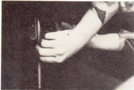
Under-dash mounting Step 4/Mark the holes for drilling by using the bracket as a template. Hold it firmly and mark carefully.
