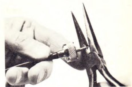
Trim the center conductor flush with the front tip of the center contact.
