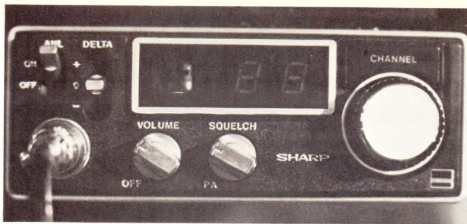
When the surrounding light level is a mite too bright, channel numbers made of illuminated line segments can fool you. Mount your mobile under-dash for maximum shading.
