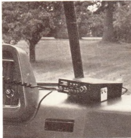
Dash-top mounting won't obstruct vision from the driver's throne in this motor home. But don't leave a goody like this Kris XL-23 where CB snatchers can window shop.
