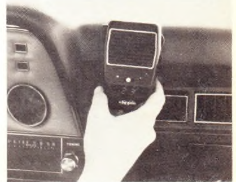
Trunk-mounting Step 13/Locate the remote-control head high on the dash where you can see the indicator and hear the built-in speaker. This dash is padded, so I'd glue on a pair of Velcro tabs for a mike hanger.
