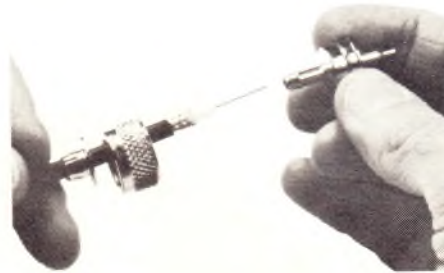
Slide connector body over the center conductor.
