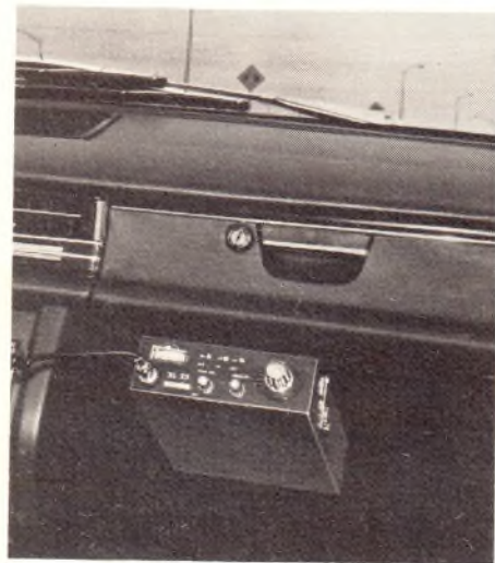
The most popular location for add-on CB installations is under the dash. You should be able to reach it without leaning over or taking your eyes from the road for more than a second or two.
