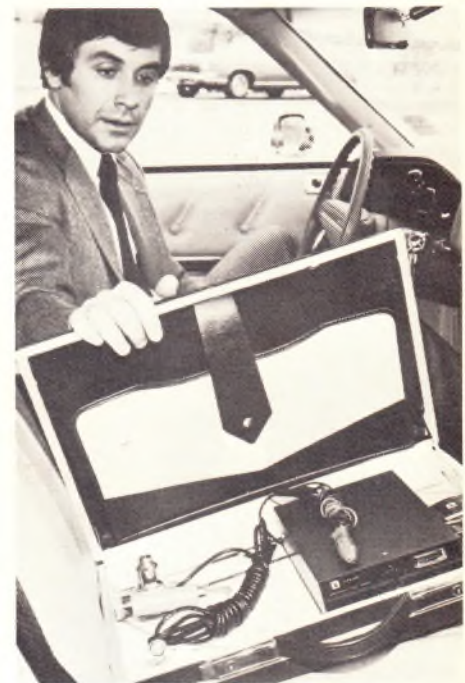
An attache case is a good way to carry your set around without being obvious. Handy for travelers and car renters, this case holds a Johnson Messenger 123A transceiver and an Antenna Specialists magnetic-mount whip.
