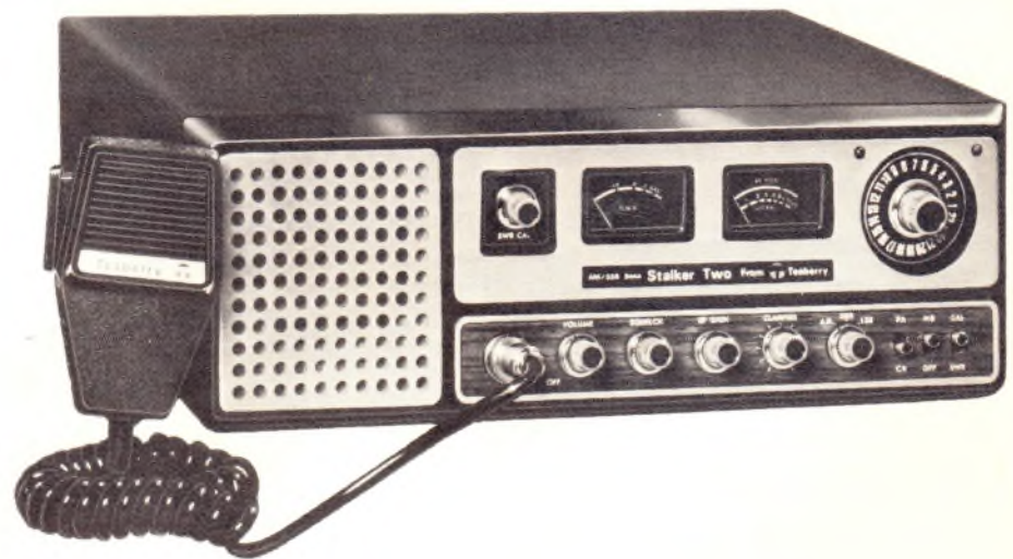
Serious Cbers head for the sidebands when they put in base stations. This is Teaberry's Stalker Two with the rock-steady phase-lock-loop which is best for SSB.
