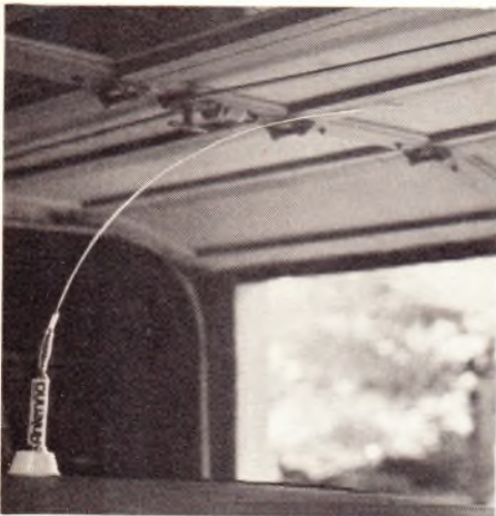
Center-roof mounting gives a nearly omnidirectional pattern. This magnetic base mount by Antenna, Inc. adheres to vinyl-topped metal roofs. I tested it against my garage door and at high speeds.
