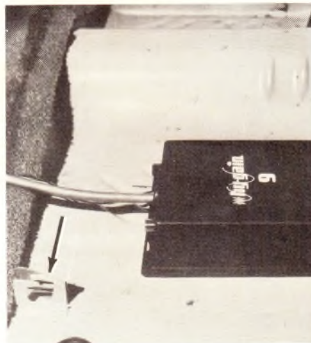
Under the front or back seat is a good location for a remote-control set such as this HY-Gain 9. Notice the seat clip (arrow). To remove seat, you have to defeat these little clips.
