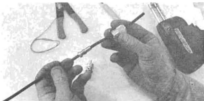
Slip adaptor and outer cylinder over cable.
