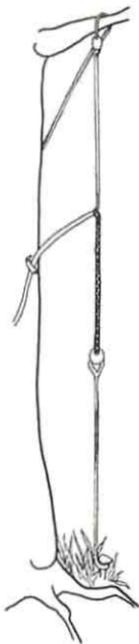
Just attach a coax connector on the end of the coax going to your transceiver and you're on the air. The SWR should be 1.5 or better, if cut to the proper length. It'll get out about as good as a  $\frac{1}{4}$  wave ground plane antenna if you get it up high and in the clear. Don't hoist this antenna up next to a metal pole, because the metal will interfere with the antenna's operation and make a high SWR.
