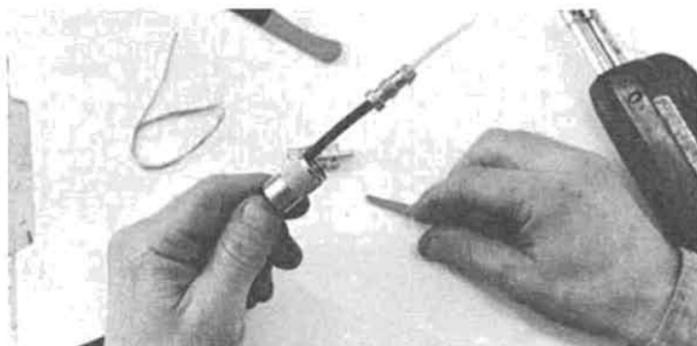
Slide adaptor up to end of black outer insulation and bend the shield down over it. Then cut the shield so that it doesn't extend down over the threads of the adaptor. (RG8 is larger than RG58 and does not require an adaptor. The braided shield is folded back on itself.)
