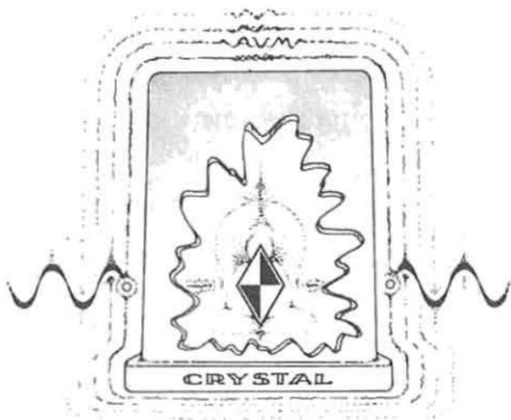
A crystal is just what it says. It is a piece of quartz crystal (a "rock") in a can. It operates on the same principle as a tuning fork. When you hit a tuning fork, it will vibrate at a particular frequency. The tone or frequency depends on how the tuning fork is constructed. A crystal operates in a similar way. When hit with the application of electricity, the crystal will vibrate at a frequency. Depending on how the crystal is cut, the frequency will vary.
