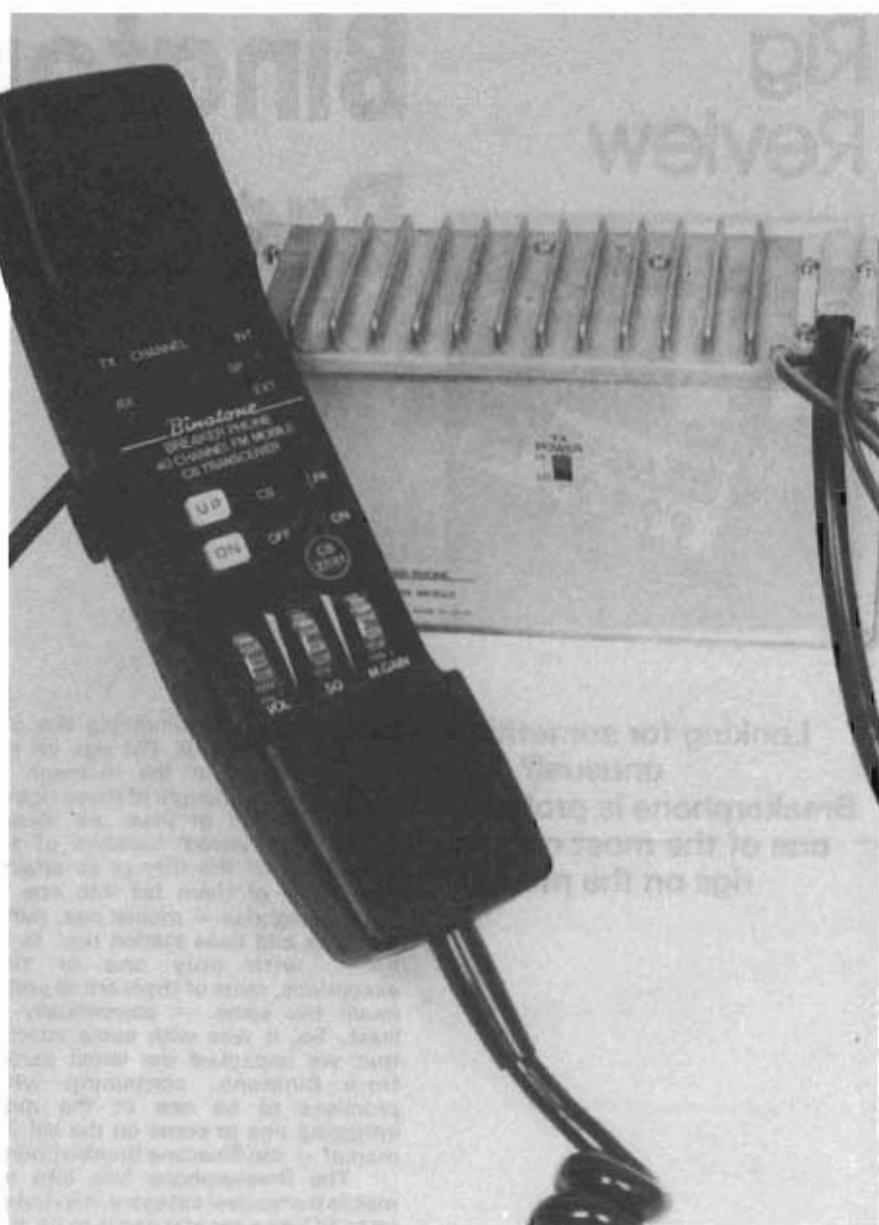
Above: Note the Hi/Lo attenuator switch on the main unit.
