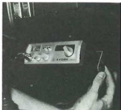
Fixing the rig to its mounting bracket.
