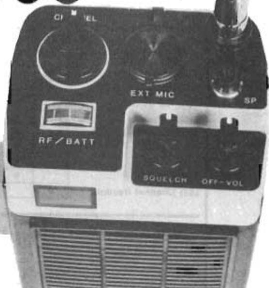
First, the 1001 has a full range of input and output sockets, including antenna, mike, power, ex speaker and DC charger. Put another way, the 1001 can be used in literally any situation — from simple hand-held portable to full system mobile to static base operation, just by plugging in the appropriate selection of antennas, mikes, speakers and power connections.
