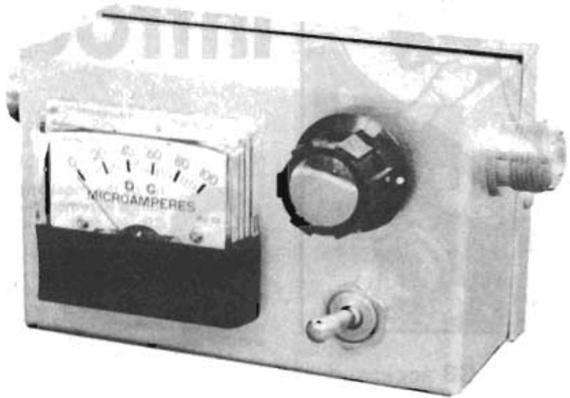
SWR meters are essential for efficient CB operation. We have a design for what may be the simplest SWR ever. It can be built in an evening and should cost significantly less than commercially built models
