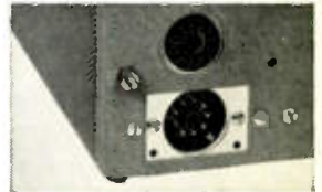
ACCESSORY SOCKET on rear panel (above power cord receptacle) for instant attachment of "Tone Alert"
