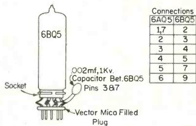
Install a .002 1KV disc capacitor between lugs 7 and 3 on the socket. Use plastic sleeving over the leads and keep the leads as short as possible. The unit is now complete.
