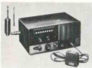
The crystal chamber has also been modified and the HE-15B now has eight switch selected transmit crystals all accessible through a slot in the front panel.
