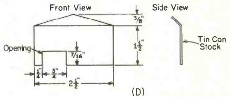
These illustrations show the mechanical details of the preamp. Diagram (A) shows the mechanical specifications and layout of the chassis. (B) shows the dimensions of the removable cover. (C) indicates the proper layout of the parts through the punched holes of the chassis. (D) indicates the dimensions and proper preparation of the internal shield which goes beneath the chassis.
