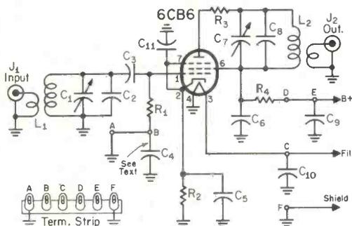
The schematic of the S9 Preamp, showing the connections to the terminal strip.
