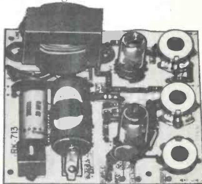
Printed circuit kits such as Allied Radio's "Knight VTVM" have most of the components, including tubes and transformers, mounted on a PC Board. The component leads are inserted into the indicated holes and then soldered in place. The board is then mechanically secured and connecting wires complete the instrument.
