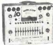
Dynamic Conductance Tube & Transistor Tester #666
