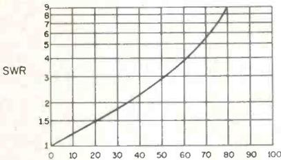
This graph shows how much of your signal is reflected back into your transmitter (and therefore not radiated), as SWR rises. Some CB installations have been measured as having an SWR rating of 7:1, indicating that about 75% of the potential signal was being wasted.
