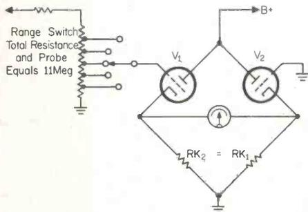
If V2's grid is connected to a positive voltage (through the divider) the current through V2 increases. The increased current increases the voltage across Rk2; the bridge is unbalanced and current will flow through M causing a "reading".
