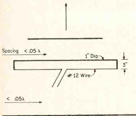
Fig. 4. Closed-Spaced Beam
