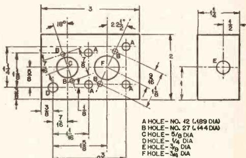
Fig. 4. Chassis layout, top view.
