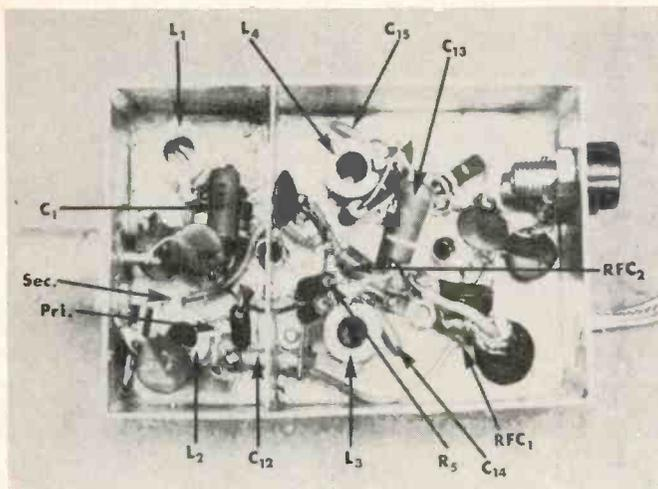
Fig. 5. Bottom view of wired chassis. Main components and their locations are identified.
