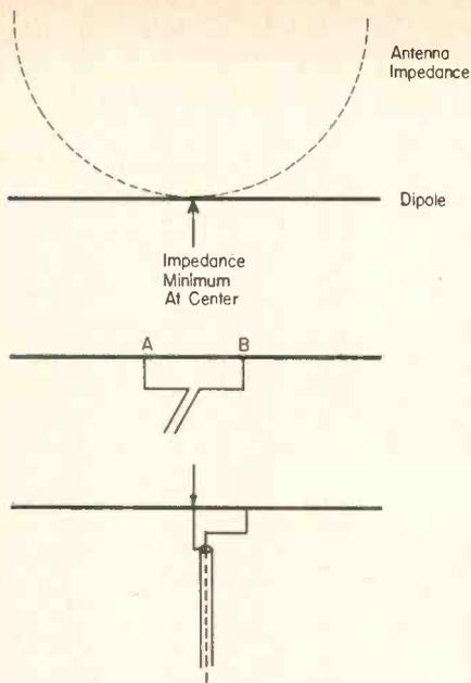
Fig. 3. The Gamma Match For A Beam Antenna
