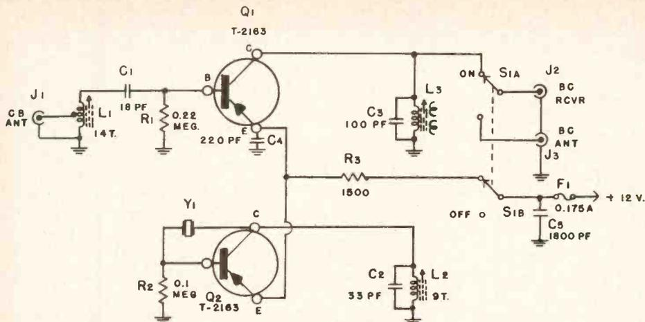
Fig. 2. Schematic diagram of 9W0831's "mini-verter."
