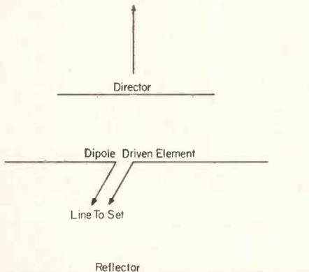
Fig. 1 The Three Element Beam Antenna
