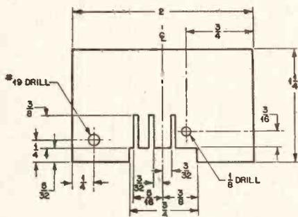
Fig. 3. Layout of interstage shield.
