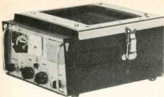
rather compact transceiver is designed and built for 15 watt operation although it has been factory pre-set for the legal five. The use of high rated components that are operating far below their maximum capability results in greatly extended operating life with relative freedom from repairs.
