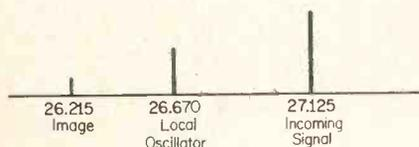
Fig. 2. The use of "heterodyning" in a CB receiver.
