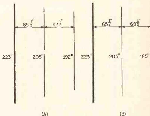
Fig. 2. Beam Antenna Dimensions
