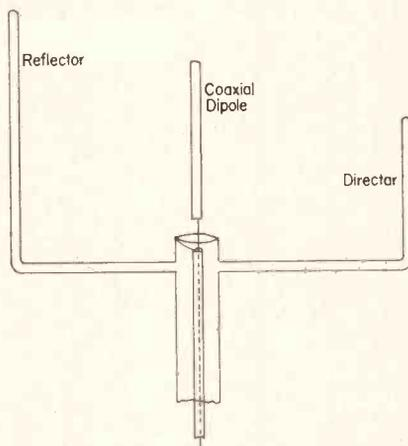
Fig. 5. Vertical Beam Antenna With Coaxial Dipole
