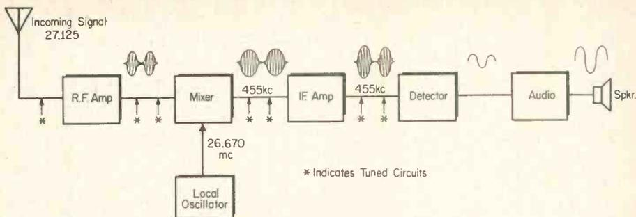
Fig. 1. Block diagram of a typical CB receiver.
