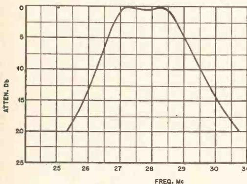
Fig. 2. Overall response of preamp.
