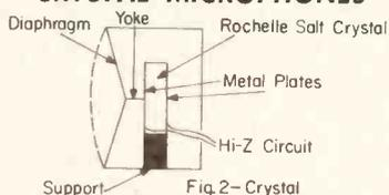
Pierre and Marie Curie (of radium fame) discovered that quartz, when subjected to physical strain produces an electric potential. This so-called piezo-electric effect is also characteristic of other types of crystals. In commercial crystal microphones Rochelle
