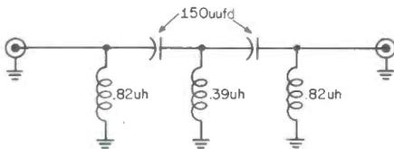
The circuit shown in the accompanying diagram is just such a filter. It consists of two 150 mmfd capacitors, two Miller type 9230-18 chokes, and a Miller type 9230-10 choke.
