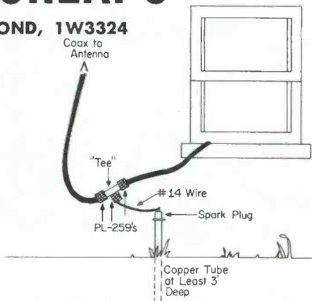
tom of the spark plug snugly into the top end of the tube (make sure that the tubing you use is of sufficient diameter to receive the spark plug). The final connection is when you place the free end of the No. 14 wire to the top of the spark plug.
