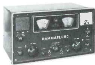
With one unit you get both Ham and CB coverage—and can listen to short wave stations all over the world. This is a quality communications receiver with a built-in 5 watt transmitter—which can easily be retuned for 10 meter use when you get your Ham ticket.
