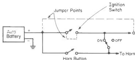
It's one thing to get your mobile rig stolen, but it's another thing when the car is still attached. The easiest method (and most commonly used) is to short circuit the ignition switch with a piece of wire.
