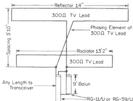
My computations determined that the reflector length (computed for the center of the band) should be 14 feet, the radiator 13 feet 2 inches, the spacing between elements 3 feet 10 inches, and the matching balun (to convert the 300 ohm antenna impedance to 75 ohms for use with coax) length 9 feet.
