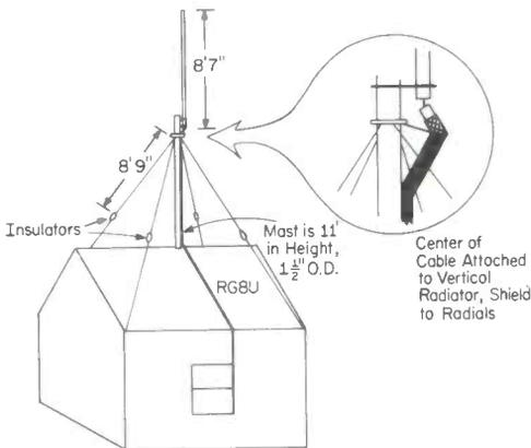
Instead of an actual whip, you might try using a length of 1/2-inch aluminum electrician's conduit, or, for a little more money, the same size tubing made of the stiffer alloys of aluminum.
