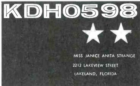
A line negative used for the contact printing of postcard QSL's on sensitized stock.
