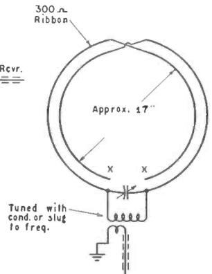
Clip free ends (marked X) until loop tunes to frequency.
