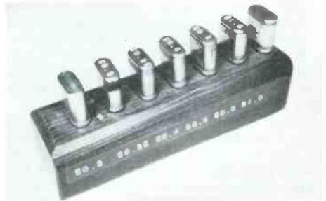
The Rock Rack is merely a short length of 1 x 2 inch wood stock with holes appropriately drilled to accept the pins of the type crystal holder you use. Most CB crystals are of the HC/6U type with .050" pins spaced .486" apart, although some have fatter pins (.093").
