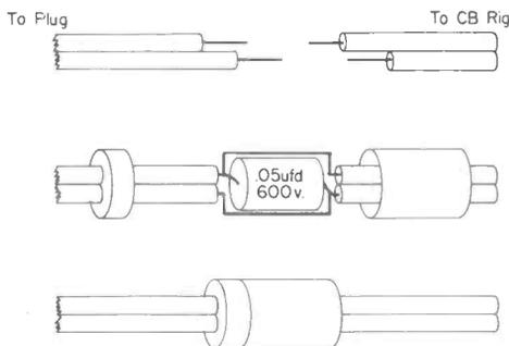
of those cylindrical plastic pill bottles which most drug stores keep in stock. A hole is drilled in the bottom of the bottle and also in the cap and these are placed on the power lead before the capacitor is connected. The bottle must be at least 1" long by 1/2" in diameter to enclose the capacitor.
