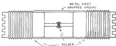
The connection of two or more lengths of RG-58/U or RG-59/U coax frequently becomes necessary and requires the use of a PL-275 straight through adapter which can be difficult to procure on short notice, and costs about \$2.30 when you do find one. Chassis type receptacles, SO-239, are usu-
