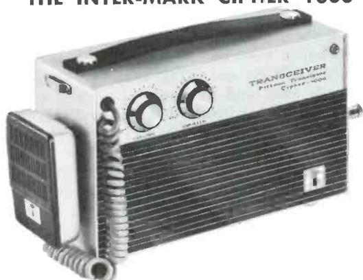
This month we put the Inter-Mark Cipher 1000 through its paces in the S9 Lab. The rig is a portable Class D unit which is operated from 18 volts worth of flashlight batteries or from an external AC power supply (optional accessory).
