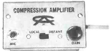
The Comtran Model C-II Compression Amplifier is a neat and small self-powered unit. Mic jack is at the left with the output gain control at the right. The LOCAL-DISTANT switch at the center cuts the amplifier in or out of the microphone circuit. The output cable with plug is for insertion into the mic jack of the transmitter.
