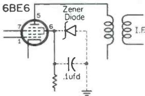
Fig. 1. Receiver drift cure for tunable units. Added circuit is shown in dotted lines.
