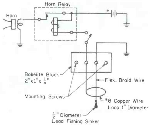
In effect, your car will "holler" whenever it is touched, even slightly, with the horn beeping on and off as long as the weighted pendulum continues to swing and bounce against the copper ring.
