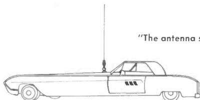
"The antenna should be in the center of a large expanse of metal"
