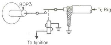
(this may be marked "horn" or "high beam"). Using coaxial cable again, with the outer shield braid firmly grounded, run a lead from the relay arm ("battery" terminal) to the transceiver's DC-power input.
