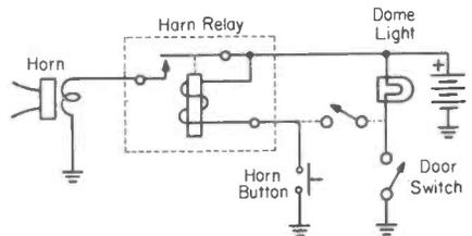
going to the horn on it. The other outside terminal will have a thin wire which goes to the horn button. The center terminal is the common one, with a heavy lead going to the battery. If you can't find the horn relay in your car, ask any auto mechanic to point it out to you.
