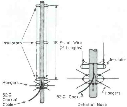
Fig. 2. The COAT HANGER KID'S antenna.
