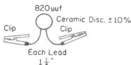
To check the possibility of fenders, body panels, mufflers, etc., introducing noise, use the portable bonding strap shown here. Attach one clip to the suspected panel or metal object and the other to the frame, making certain that both bite deeply into raw metal rather than into rust, undercoating, or dirt. Again, if the noise is reduced, make the installation permanent with sheet-metal screws instead of the big clips, and move the checking strap to another location.
