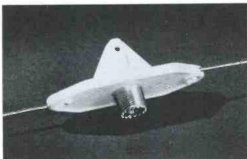
A rugged, specially-designed fitting for connecting a coaxial feedline to antenna elements now is available from Budwing Mfg. Co., P.O. Box 97, Ramona, Calif. The molded plastic and metal fitting features holes at both ends for element tie points, and has molded-in copperleads for electrical connection to an SO-239 connector.
