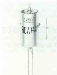
The cavity (tuned circuit) is built around the tube. For operation, it is only necessary to apply the correct voltages and connect an antenna. Type 7533 is used in radio-sondes for weather observations; other versions are ideally suited for a variety of compact applications, such as in aircraft identifiers and high-way traffic radar equipment. Price: \$7.00-\$60.00.
