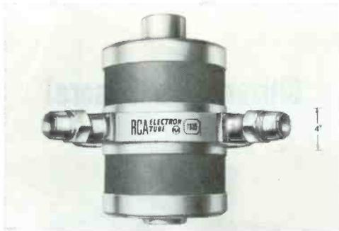
ful AM broadcast stations) and millions of watts of pulse power. Widely used in long-range radars, space research, and nuclear particle accelerators. Although the 3.5-volt filament voltage of the 7835 appears modest, the filament-current rating is a whopping 6600 amperes—more than 2300 watts for the filament alone. Price: \$7800-\$64000.
