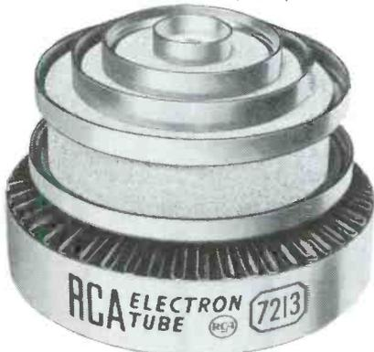
There are many families of tubes within this classification, which is flexibly defined as including tube that produce power from approximately 15 watts to 15,000 watts. Some power tubes will be found on either side of this range. Generally, these tubes perform much the same function as the rf amplifier tube in your CB rig. Cost and size are closely connected with power-handling capability and frequency of operation. Price: \$2.50-\$2000.
