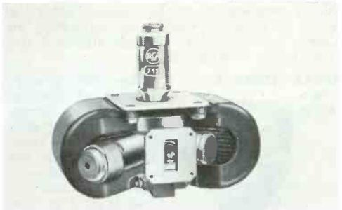
The majority of airborne radar equipments use tubes of this type to generate the high-power signal required. Magnetrons are extremely efficient generators of radio-frequency power above 500 Mc. Type 7111 can produce a minimum peak power of 200,000 watts in the frequency range from 8500 to 9600 Mc. Price: \$700-\$1200.
