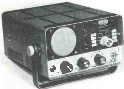
Sonar Radio Corporation, 73 Wortman Ave., Brooklyn, N. Y. gave S9 a scoop on announcing their new *Model H* which is to sell for \$159.95 (list). The *Model H* features a transistorized power supply, 7 transmit/receive channels with external sockets for transmit/receive crystal, it has an adjustable squelch and a fine tuning control for the receiver.
