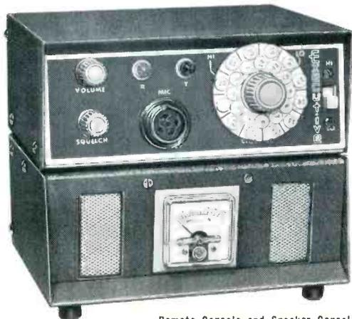
Remote Console and Speaker Console. Two units may be "stacked" or installed separately.
